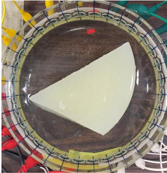
Fig. 6.4.4: phantom tank with  $1/8$  normal saline conductivity agar gel and  $1/4$  normal saline background.
