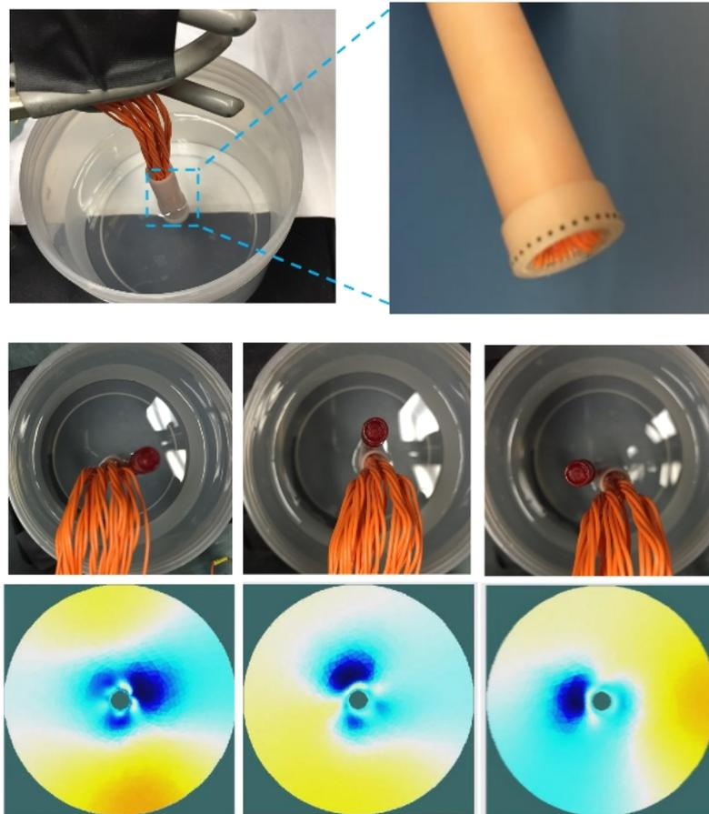
Fig 6.4.1: Top left: electrode in saline. Top right: electrode zoom-in view. Middle row: “pen in saline” experiment setup. Bottom row: reconstructed images corresponding to pen location.
