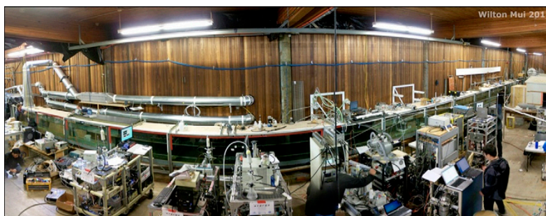
Fig. S1. Birds-eye lens view of CAICE intensive campaign conducted at the ocean-atmosphere wave flume ( 33 \times 0.5 \times 1 m) facility developed in phase I (November 2011).
