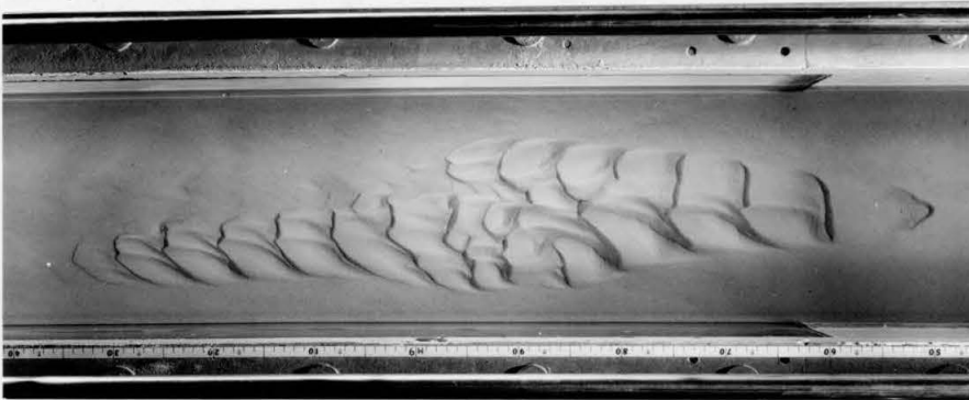
(b) Spontaneous Ripple Train at Flume Station 9.0 Formed in Approximately 2 hours. (Photo No. 11219)
