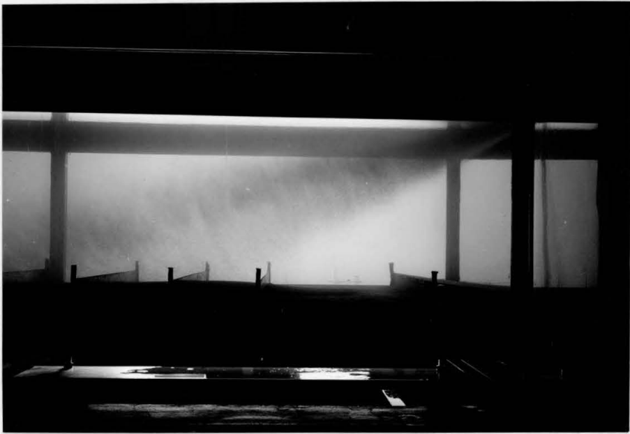
Fig. B.2 Sand Plume Which Obtained For Hopper Discharge of Approximately 60 lbs of Sand per hour; U \sim 12 cm/sec, H \sim 56 cm, T \sim 21^{\circ}\text{C} . (Photo No. 11217)
