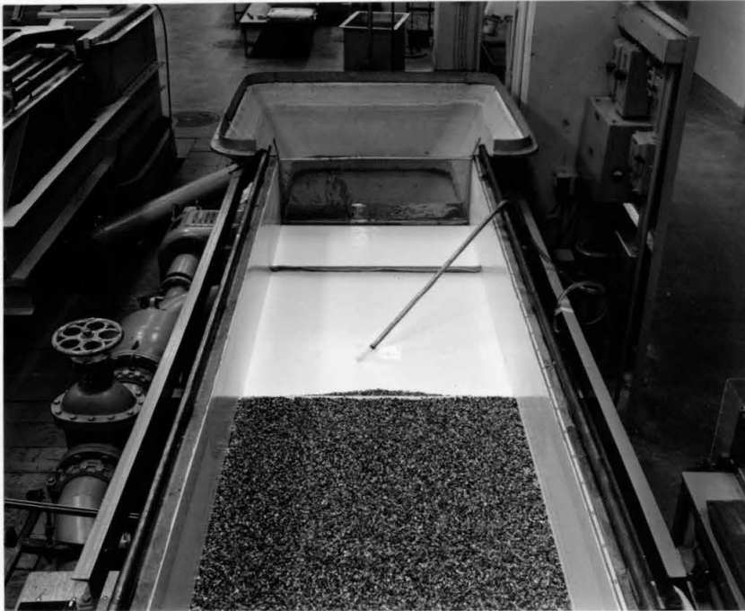
Fig. 3.8 Downstream End of 60-ft Flume Showing Slot Used To Catch Load in Series E. Siphoning tube to remove load samples is also shown. (Photo No. 11206)
