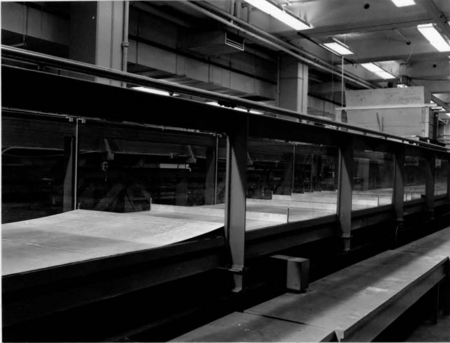
Fig. B.1 Upstream View of 130-ft Flume With Metal Hopper Mounted on Side Walls, And Metal Slot Dividers Positioned on Flume Bed. Note metal sheets which provided smooth transition from tops of end slots to flume bed. (Photo No. 11216)
