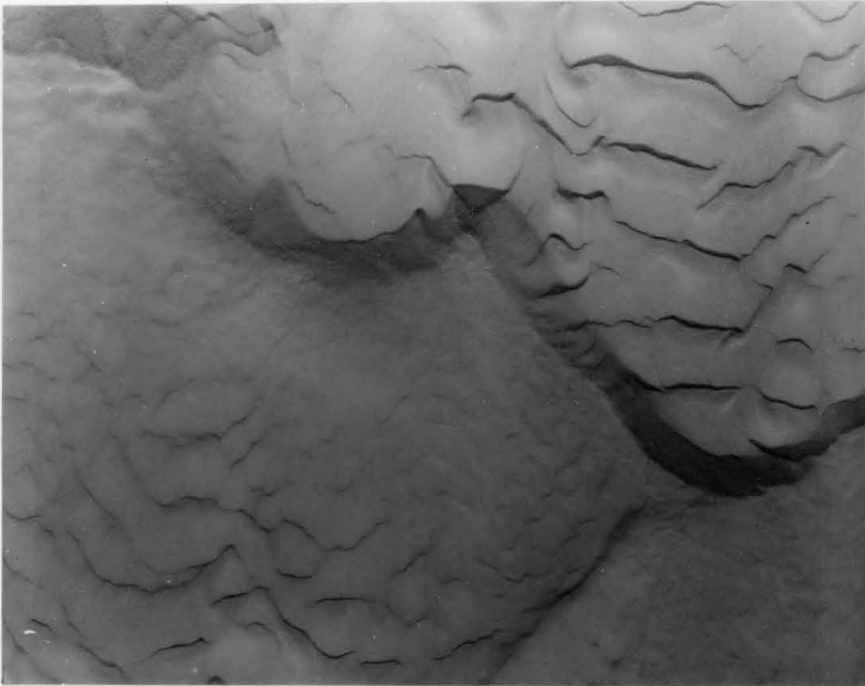
(b) Typical Dune Front in F-34 ( T \sim 38^{\circ}\text{C} ). (Smaller ripples on bed were formed during flume shutdown, Photo No. 11215.)
