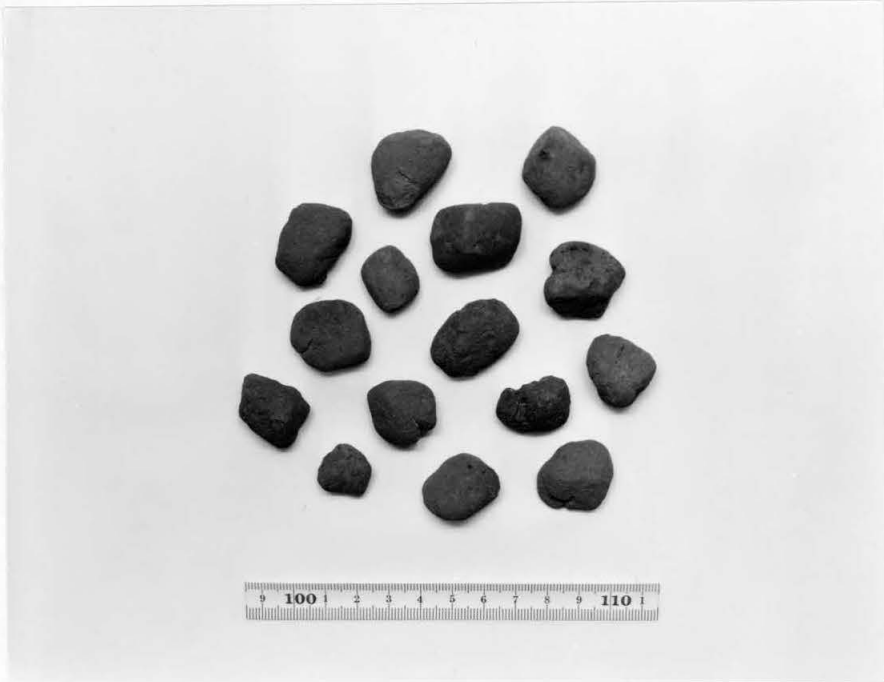
Fig. 3.18 Sample of Coarse, Synthetic Clay-Aggregate Particles Used in Series D. (Scale is in cm, Photo No. 11211)
