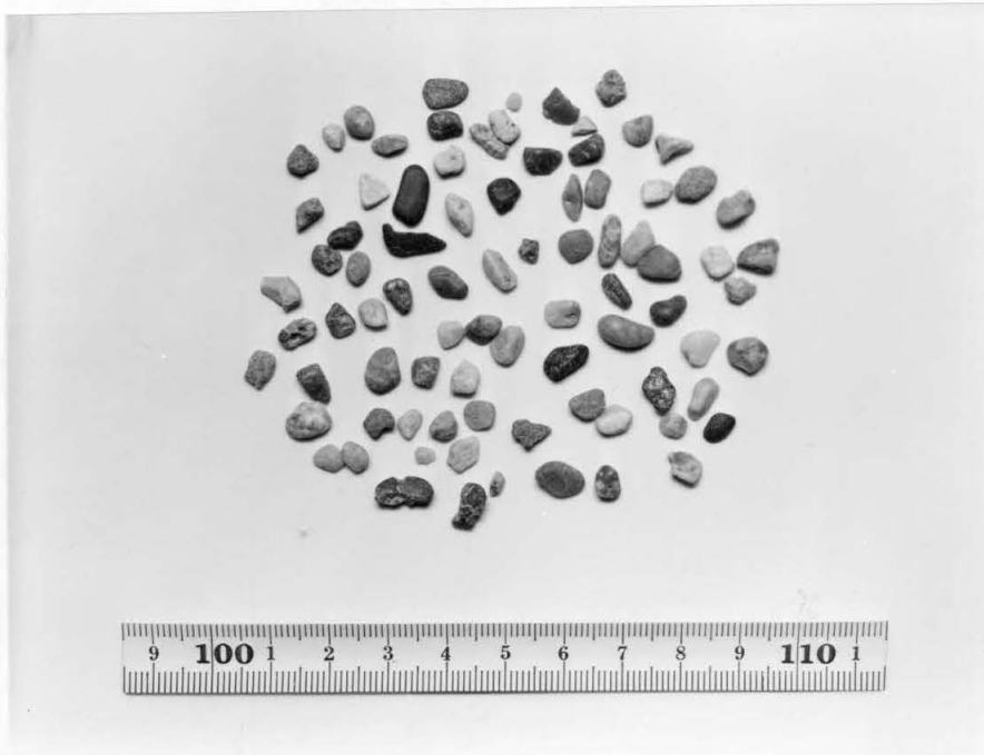
Fig. 3.19 Sample of Fine Gravel Used in Series E. (Scale is in cm, Photo No. 11212)
