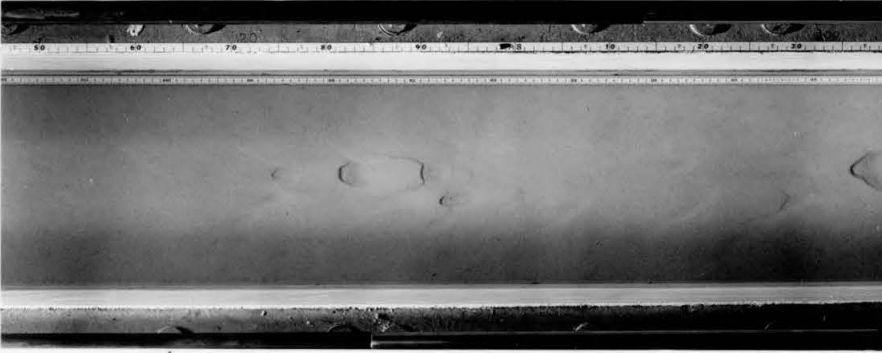
(a) Spontaneous Ripples Near Flume Station 8.0 (8.0 meters below inlet) Formed After 1-1/2 hours. (Photo No. 11218)
