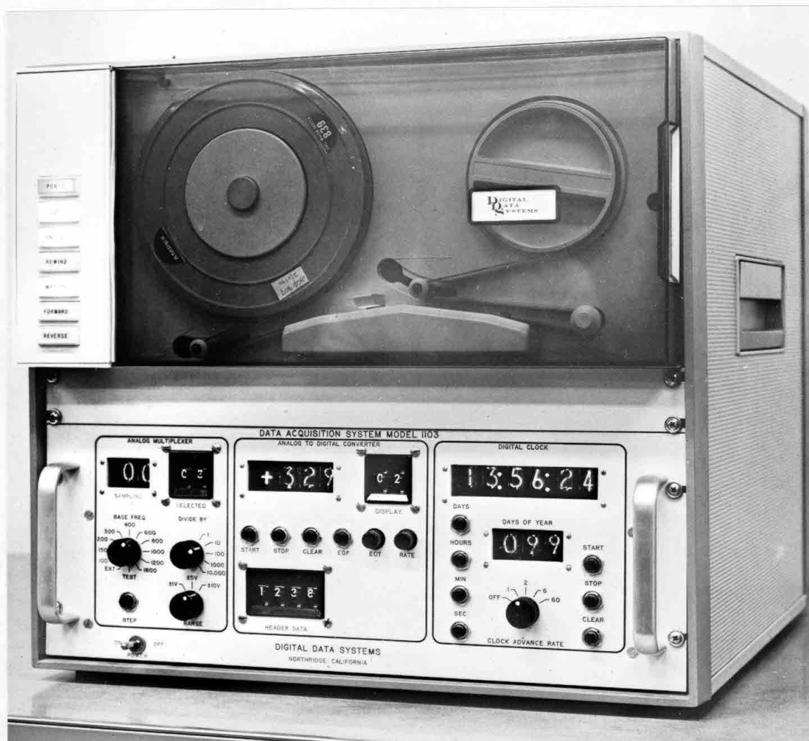
Fig. 3.12 Data Acquisition System Used to Digitize Analog Bed Profiles, and Store Digitized Output on Magnetic Tape. (After Okoye (1970))
