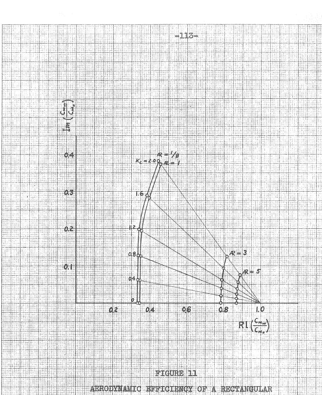
AERODYNAMIC EFFICIENCY OF A RECTANGULAR OSCILLATING WING AT N=10/7, (B) Cm,/Cm.
