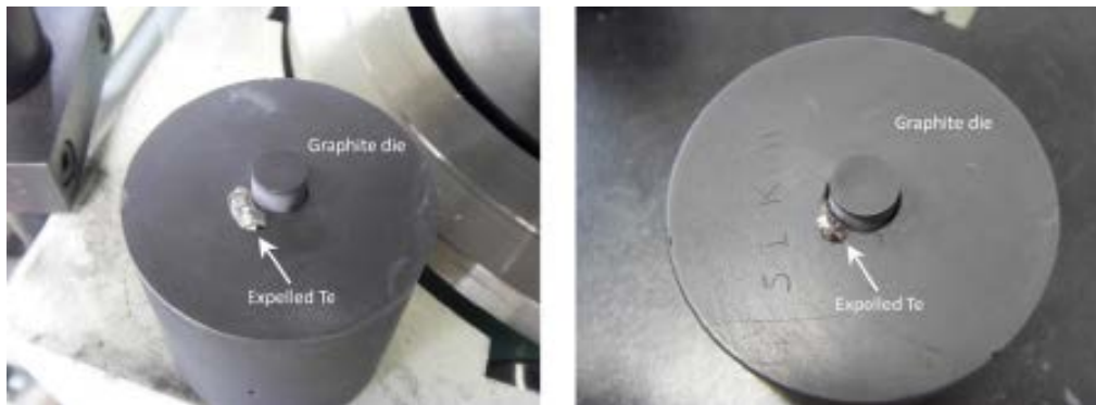
Fig. 2.5. Picture of excess Te expelled from the graphite die after the SPS process.
