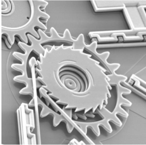
Figure 1-3: a MEMS device with micro mechanical gears ([www.thenanoage.com](http://www.thenanoage.com))
