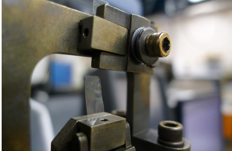
Figure 2-3. DMA setup for tensile test of PA-C film. Shown in the figure is a 200°C pre-annealed sample but broken after the tensile test.
