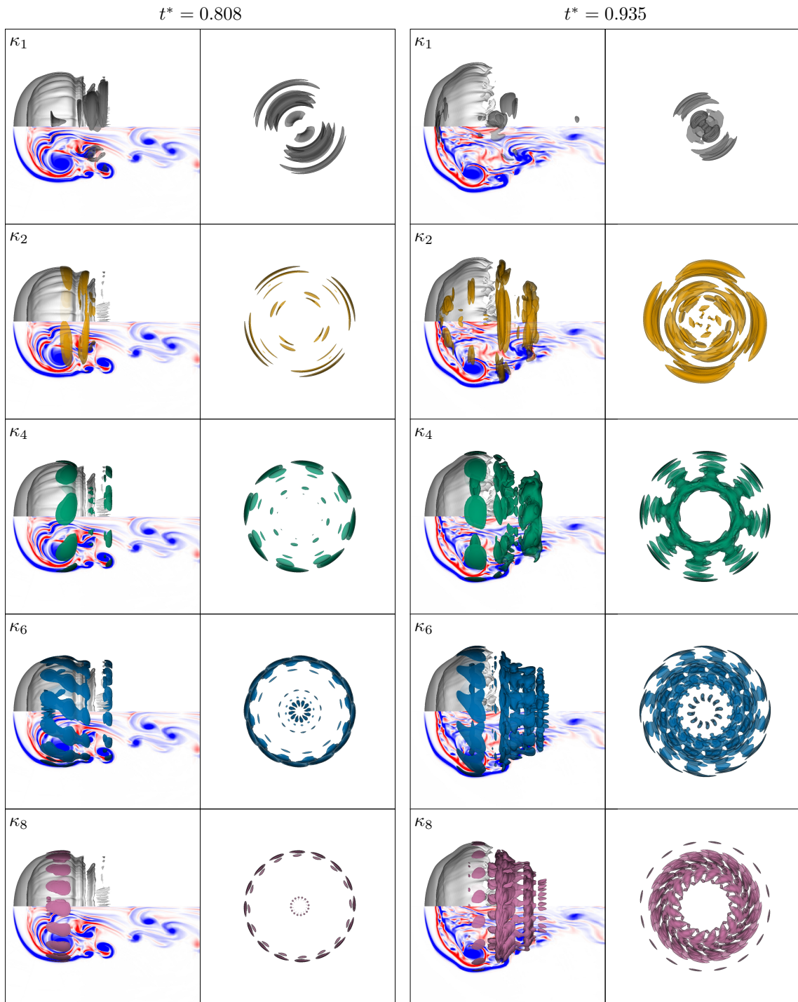
Figure 6.17: Isosurfaces of \kappa_m , m = 1, 2, 4, 6, 8 at t^* = 0.808, 0.935 . Also shown is the liquid sheet visualized using \alpha_l = 0.01 , and a filled contour slice of azimuthal vorticity. Front and side views are shown, and isosurface values change between frames.
