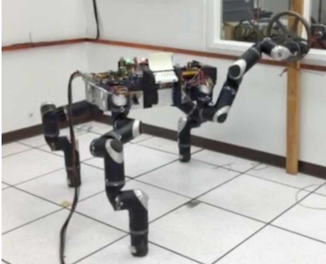
Figure 5.1: Photograph of the Four-Limbed RoboSimian Robot used by the JPL/Caltech team in the DARPA Robotics Challenge. This snapshot shows RoboSimian turning a circular valve on the vertical wall in the background using one of its limbs, while maintaining quasi-static stance stability using its other three limbs. Because the robot did not have hands mounted at the time, it needed to maintain a normal inward force, while moving around the axis of the valve.
