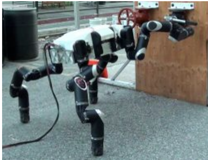
Figure 3.1: RoboSimian turning a valve mounted on a wall. Designed by NASA\JPL-Caltech
