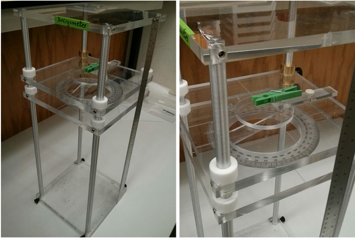
Figure 3.1: Divergometer used for measuring divergence angles and plastochon distances. Left panel shows the entire device. Right panel shows a closeup of the rotating protractor.
