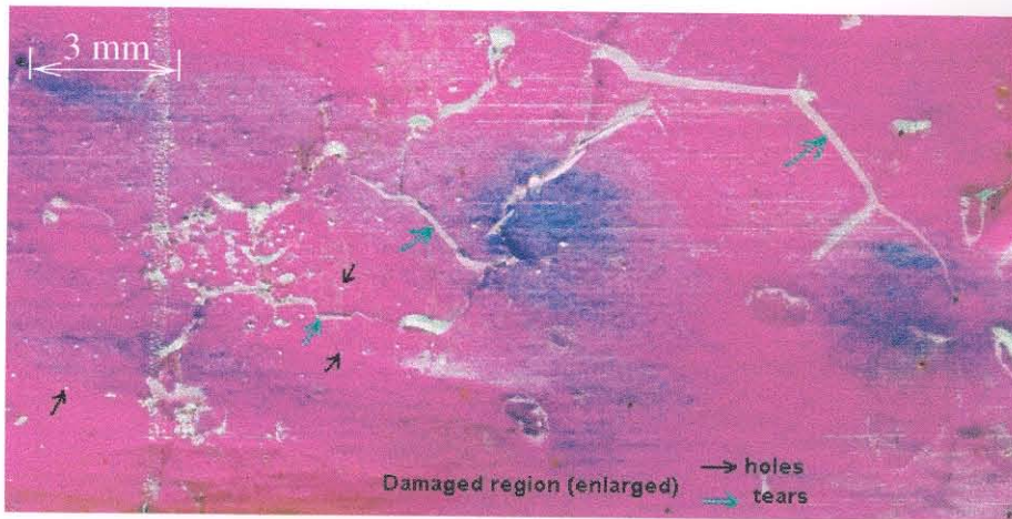
Figure 3.16: Cellophane film subjected to 50 lithotripter shocks @ 18 kV, 1 Hz. Damage comprises of holes and tears.
