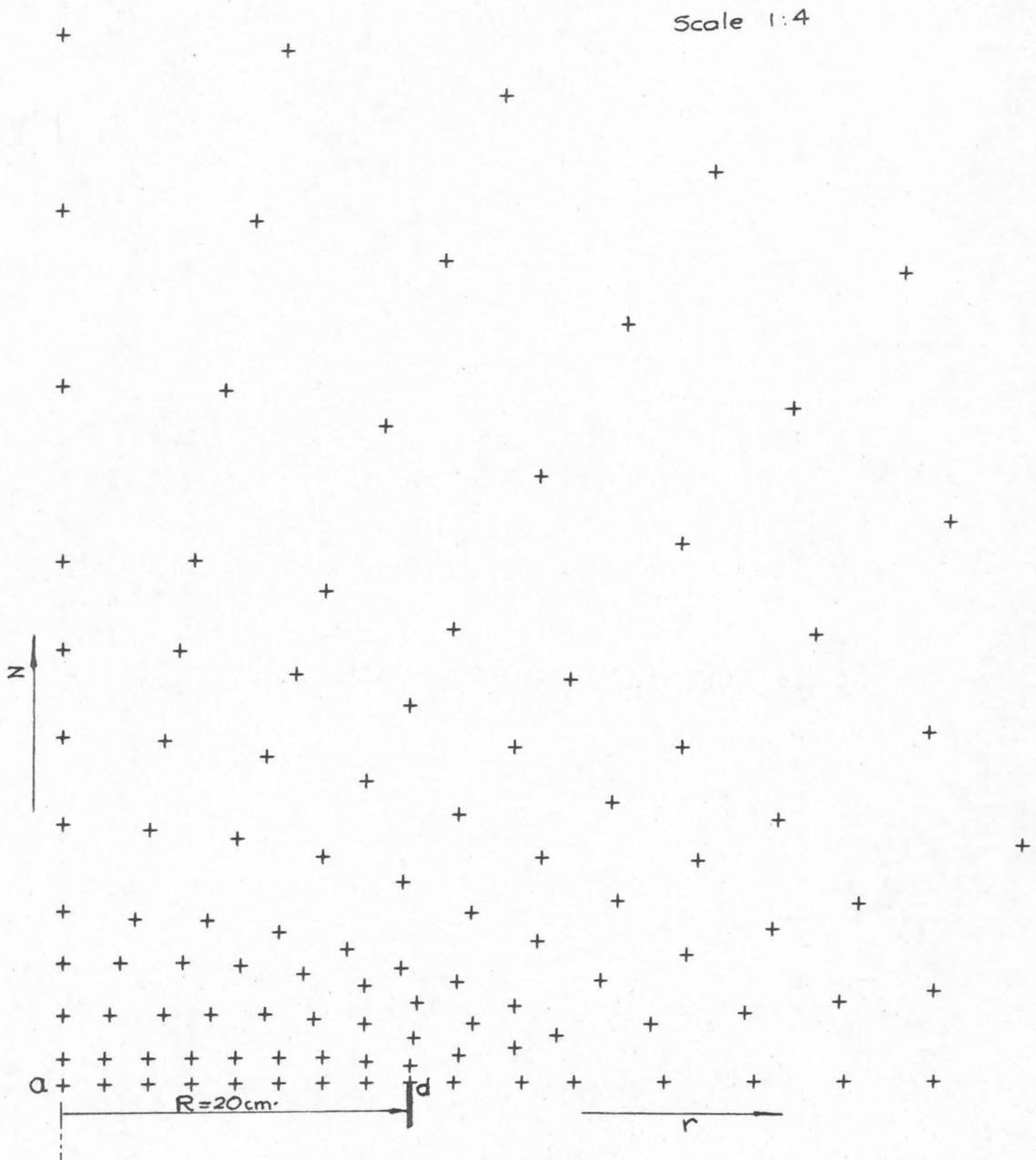
Fig. A-9. Finite element mesh near the punch surface
