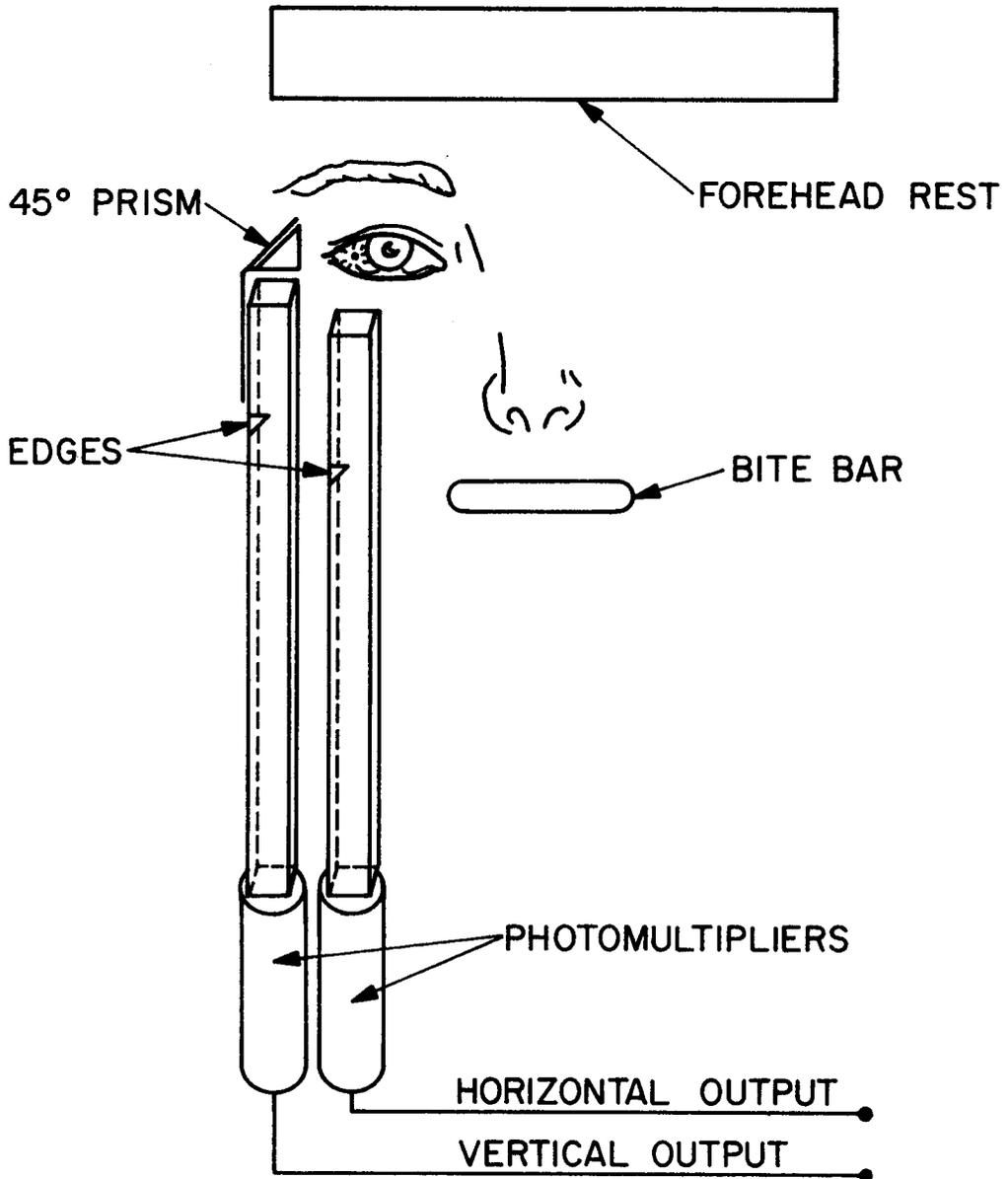
Figure 2.4: Photomultiplier tube assembly for the measurement of eye movements. The pin-light attached to the contact lens casts the shadow of the edge onto the face of the photomultiplier tube; the output of the PMT's is thus proportional to rotation of the eyeball.
