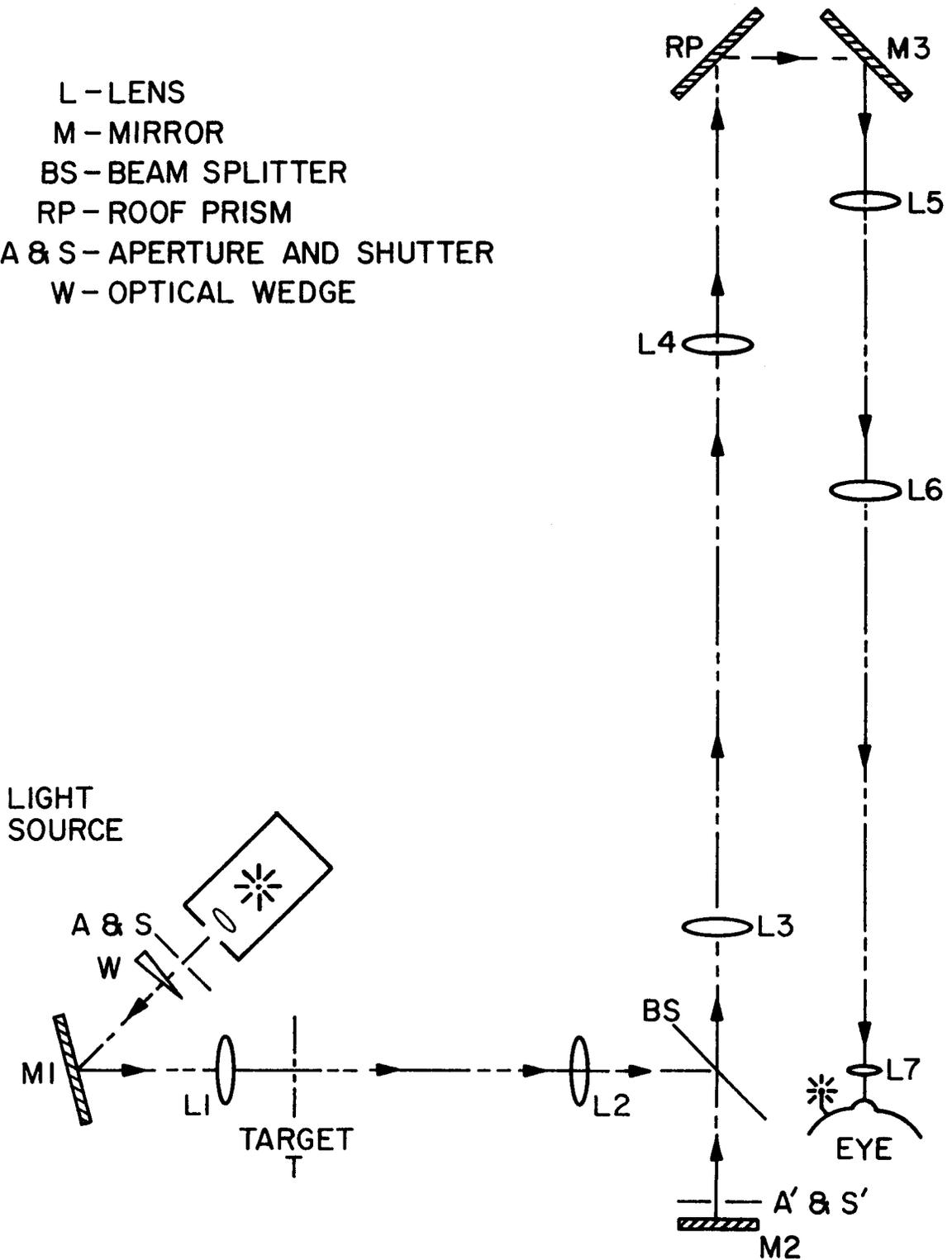
**Figure 2.5:** Optical system for the presentation of the stimuli during stationary fixation experiments.
