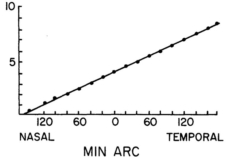
Figure 2.6: Linearity check: Amplified output of the photomultiplier tubes (volts) vs. rotation of the artificial eyeball (min arc).
