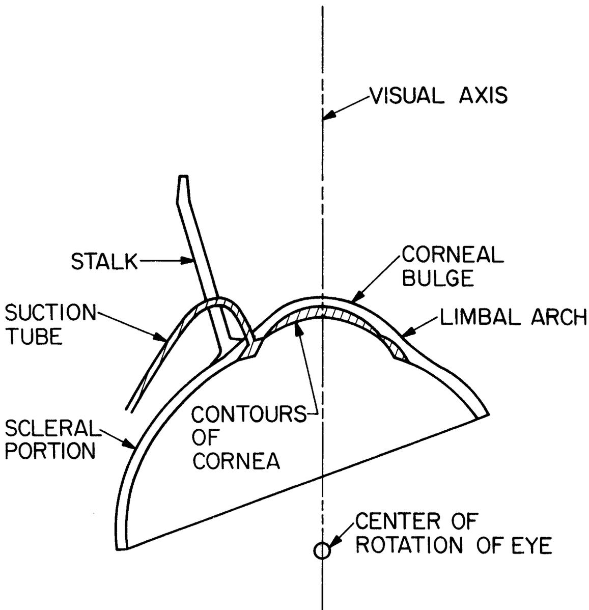
**Figure 2.2:** Contact lens worn by the subject for the measurement of eye movements (Cross section).
