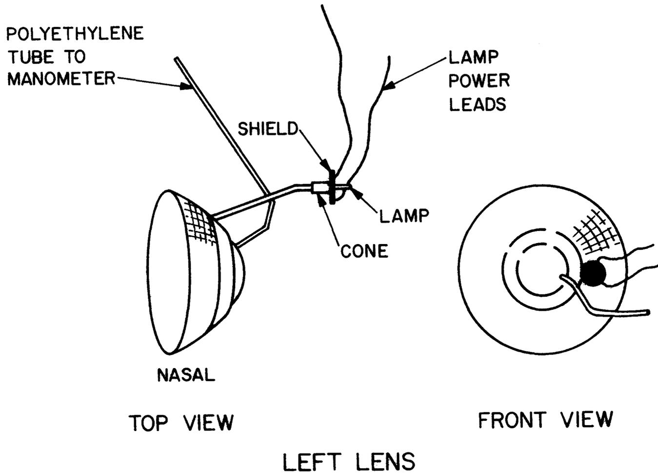
Figure 2.3: Contact lens worn by the subject for the measurement of eye movements (Perspective).
