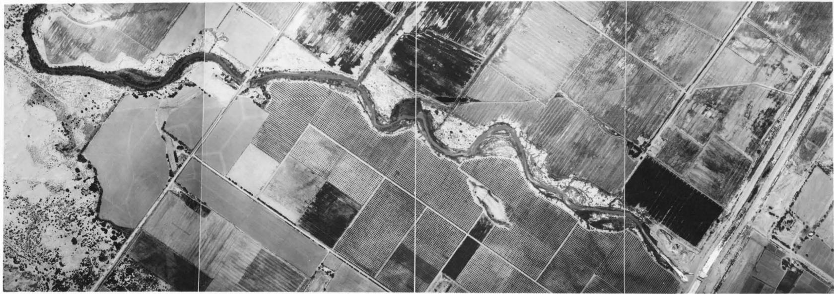
Figure 1.1b. Aerial photo of the Imperial fault taken shortly after the 1940 earthquake. The orange grove in this photograph lies south of the Cole Road near the point on the fault nearest to Bonds Corner.
