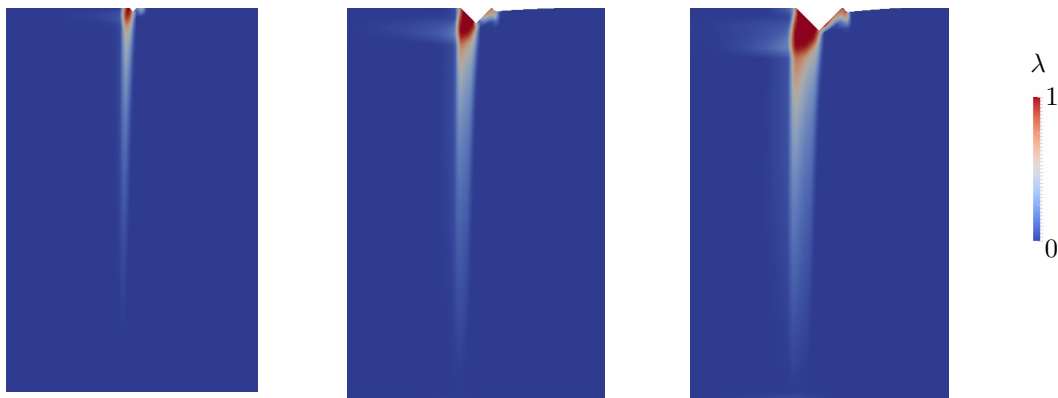
Figure 5.3: Twin evolution in terms of the twinning ratio of calcite e^+ twin for a nanoindentation test predicted by our crystal plasticity theory.
