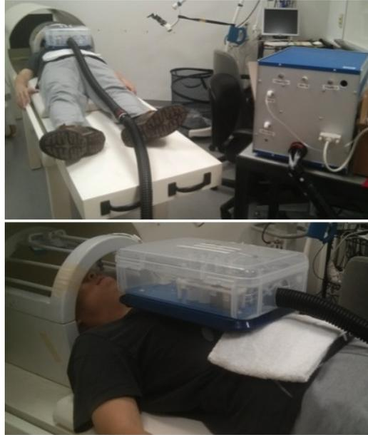
Figure 3.2: The Olfactometer Setup.
