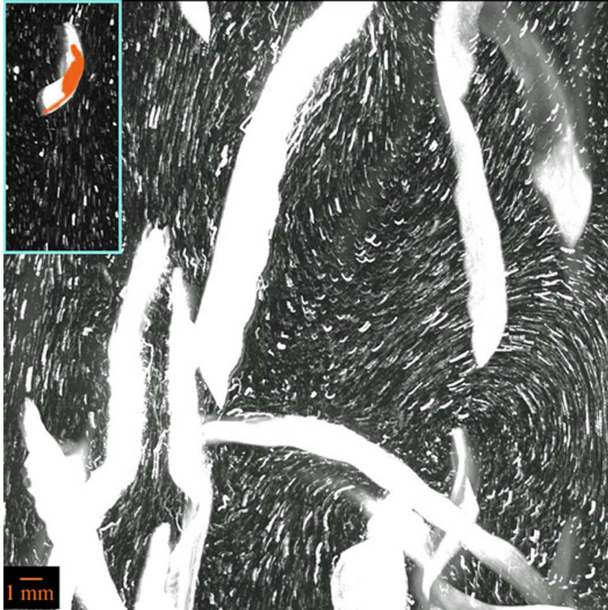
Figure 4.11: Visualization of flow pathlines. Superposition of one second of raw PIV images displays the pathlines of the flow during vertical migration of A. Salina . The white elongated shapes indicate the trajectory of the organisms. The flow generated by a single swimmer during 0.16 s is shown in the blue inset at the upper left corner of the image. The orange shadowing indicates the size and shape of the organism at a given instant. Both images are displayed with the same spatial resolution.
