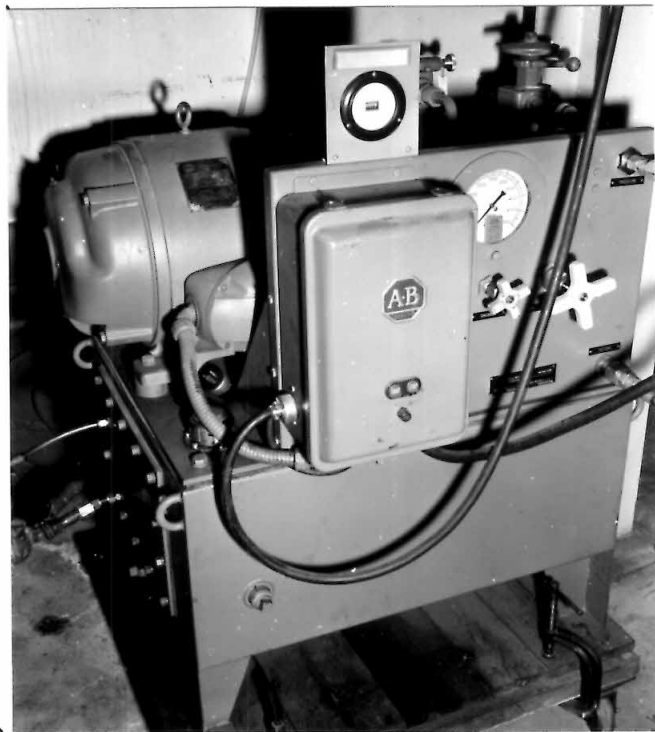
Figure 3 - The hydraulic pump and reservoir.
