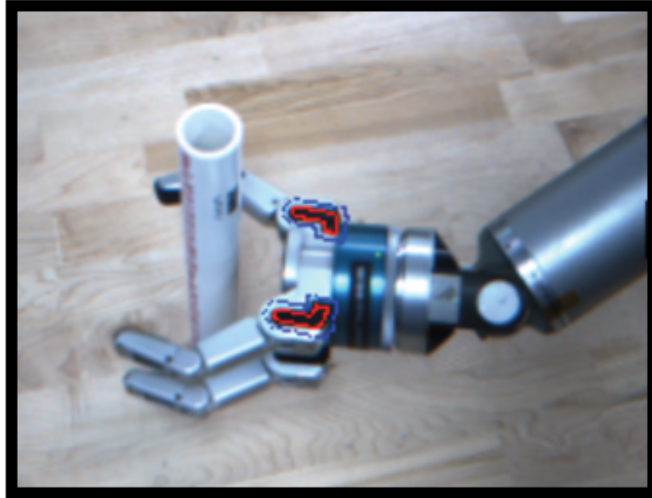
Figure 1.2: A robot arm attempts to grasp a pipe during the DARPA Autonomous Robotic Manipulation program. If the robot bumps the pipe it may fall over and roll away. Achieving a caging grasp prior to closing the gripper can guarantee that the object does not escape during the grasping motion.
