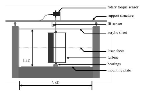
Figure 3.6: Section view schematic of the experimental setup.
