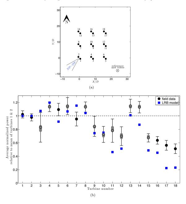
Figure 2.9: (a) Schematic of the eighteen-turbine array with the bin of wind direction. (b) Comparison of field measurements and LRB model prediction for the performance of individual turbines within the array. Error bars indicate one standard deviation.
