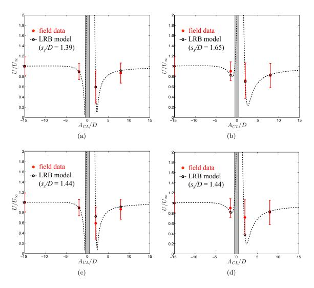
Figure 2.6: Calibration of the sink spacing model parameter,  $s_s$ . (a) Least-squares fit to the field data for the single VAWT. (b) Least-squares fit to the field data for the VAWT pair. Best fit model parameter,  $s_s/D = 1.44$ , to the combined field data for the (c) single VAWT and (d) pair of VAWTs. Open black circles indicate the LRB model prediction of flow speed at the field measurement locations. Gray rectangles indicate turbine positions.
