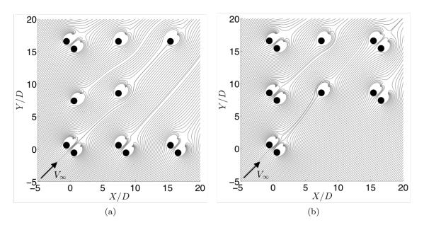
Figure 2.11: Streamlines generated by the LRB model for the (a) best and (b) worst performing arrays as predicted by the model, i.e., configuration 1 and 5, respectively.
