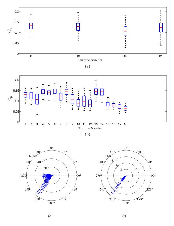
Figure 2.4: Box plot of individual turbine power coefficient (a) when four turbines are operational for all wind directions, and (b) when eighteen turbines are operational and wind direction is between  $215^{\circ} - 235^{\circ}$ .(c) Wind rose in degrees from due north for the four-turbine array, and (d) the eighteen-turbine array. Wind speeds are between 6-10 ms<sup>-1</sup> for both cases.
