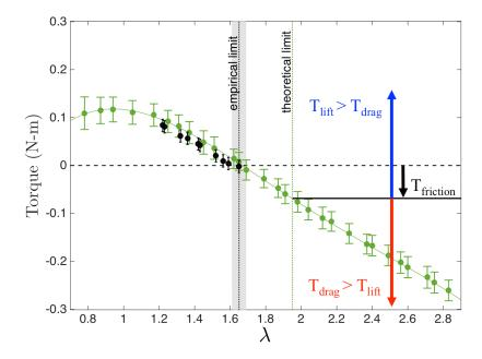
Figure 3.26: Measured torque for flow-driven (black) and motor-driven (green) cases. Error bars represent an estimate of one standard deviation in measurement error. A fourth-order polynomial is fit to the motor-driven points.
