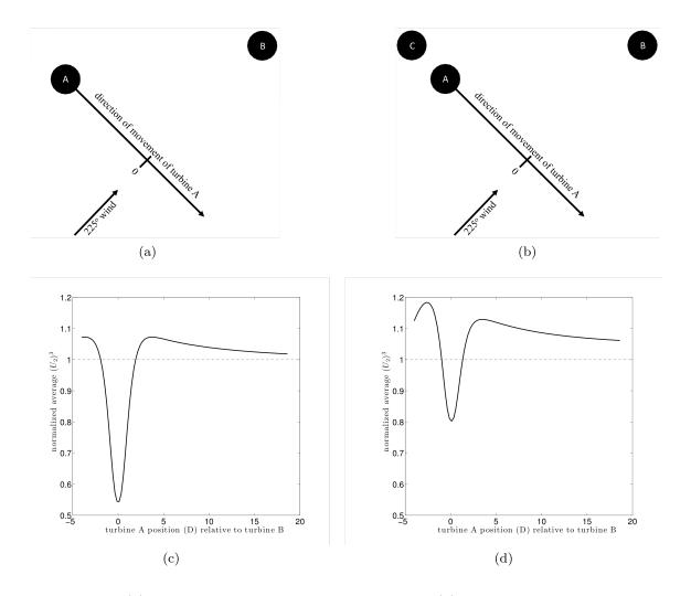
Figure 2.12: (a) Schematic for a two-turbine array and (b) three-turbine array, and the LRB model prediction of array performance for each, (c) and (d), respectively. Turbines are drawn to scale with the initial position of turbine A indicated in the figures.
