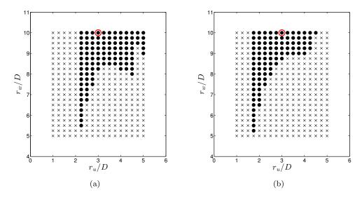
Figure 2.14: Parameter study of the LRB model prediction of array performance with varying the sink spacing,  $s_s$ , model parameter. (a)  $s_s/D = 1.0$ , (b)  $s_s/D = 2.0$ . Black circles indicate the model correctly predicts the ordering of array performance and black X's indicate where the model fails. The red circle indicates the nominal model parameters of  $r_u/D = 3$  and  $r_w/D = 10$ .
