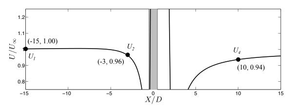
Figure 5.2: Axial velocity distribution for a single VAWT by the LRB model. Gray rectangle indicates turbine position.
