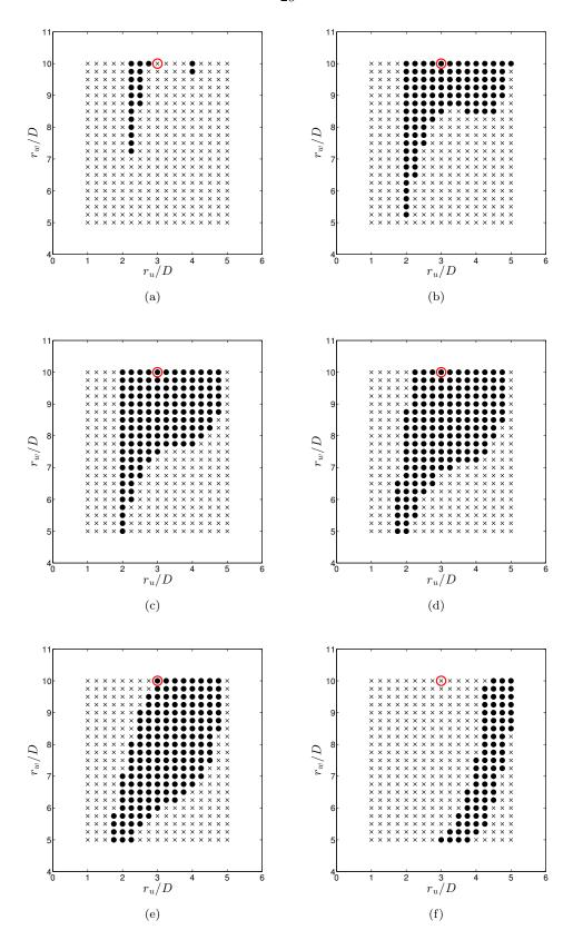
Figure 2.13: Parameter study of the LRB model prediction of array performance with varying  $C_p$  as (a) 5%, (b) 10%, (c) 15%, (d) 20%, (e) 30%, and (f) 59%. Black circles indicate the model correctly predicts the ordering of array performance and black X's indicate where the model fails. The red circle indicates the nominal model parameters of  $r_u/D=3$  and  $r_w/D=10$ .
