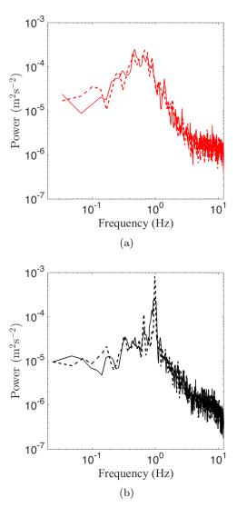
Figure 3.21: Power spectra for the spanwise fluctuating velocity component, v', in flow-driven (solid lines) and motor-driven (dashed lines) cases. Colors correspond to the nominal operating conditions on or below the neutral curve, i.e.,  $Re_D = 7.8 \times 10^4$ ,  $\lambda = 1.65$  (red) and 1.20 (black). The measured conditions for each line are given in Table 3.1.
