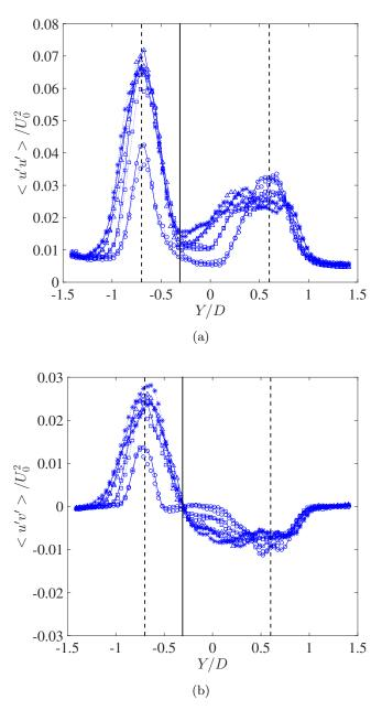
Figure 3.20: (a) Longitudinal and (b) shear Reynolds stress. All symbols correspond to those of Figure 3.19. Dashed vertical lines correspond to dominant peaks in the Reynolds stress distributions, i.e., at Y/D=-0.7 and Y/D=0.6. The solid vertical line corresponds to the minimum velocity at Y/D=-0.3
