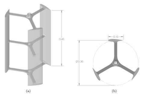
Figure 3.5: CAD drawing of the 3-bladed model turbine used in the experiment. (a) Isometric view and (b) top view. All dimensions are given in meters.
