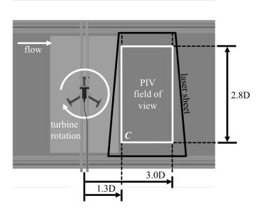
Figure 3.7: Top view schematic of the experimental setup. The contour, C, encloses the area that was used to calculate spatial averages of velocity as well as circulation. Dashed vertical lines indicate the relative position of C to the turbine center.
