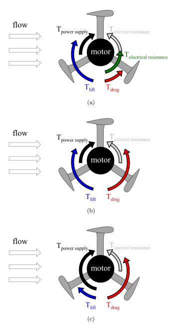
Figure 3.4: Free-body diagram of the motor-driven turbine when operating in (a) the lift-dominated regime, (b) the neutral regime, and (c) the drag-dominated regime. The components of torque that contribute to the overall shaft torque are shown in each regime with colored arrows. Note that only torques due to the motor and aerodynamics are considered, i.e., friction is neglected.
