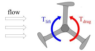
Figure 3.2: Free-body diagram (top view) of a flow-driven VAWT for the free-spin operating condition. Here the net torque due to lift,  $T_{\rm lift}$ , balances with the net torque due to drag,  $T_{\rm drag}$ .
