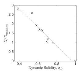
Figure 4.18: Linear correlation ( $R^2 = 0.94$ ) between the streamwise location of wake transition, i.e.,  $X/D_{\rm transition}$ , and dynamic solidity,  $\sigma_D$ .
