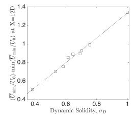
Figure 4.23: Linear correlation ( $R^2=0.99$ ) between the rescaled streamwise velocity of Figure 4.22 at X/D=12 and the dynamic solidity,  $\sigma_D$ .
