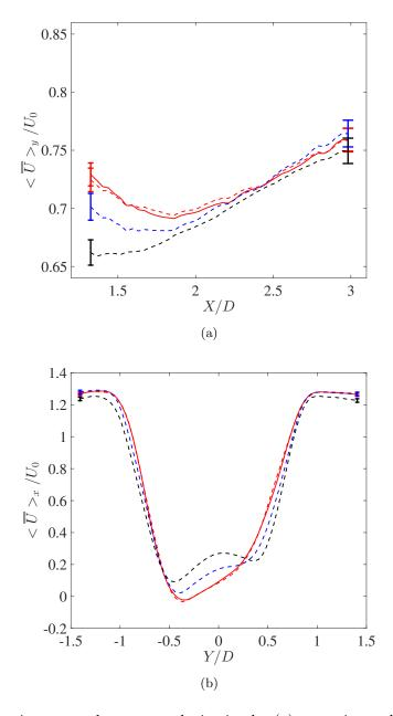
Figure 3.23: Spatio-temporal average velocity in the (a) spanwise and (b) streamwise direction when  $Re_D$  is fixed and  $\lambda$  is varied. Solid lines indicate flow-driven conditions and dashed lines indicate motor-driven conditions. Colors correspond to the nominal operating conditions on or above the neutral curve, i.e.,  $Re_D = 7.8 \times 10^4$  and  $\lambda=1.65$  (red), 1.88 (blue), and 2.02 (black). The measured conditions for each line are given in Table 3.2.
