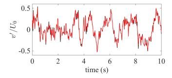
Figure 3.16: Sample of the measured spanwise fluctuating velocity component, v', normalized by the freestream velocity,  $U_0$ . The velocity sample corresponds to the point in the flow indicated by the red circle in Figure 3.15. The black line indicates the velocity as measured from PIV and the red line is the interpolated velocity used to compute the spectra.
