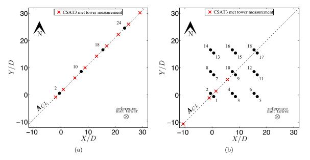
Figure 2.3: (a) Schematic top view of the four VAWT array, (b) Schematic top view of the eighteen VAWT array. VAWTs are drawn to scale with black circles and numbered individually. Velocity measurement positions are indicated by red X's. The position of the reference meteorological tower is not drawn to scale. The axis dimensions are given in rotor diameters where D=1.2 m.
