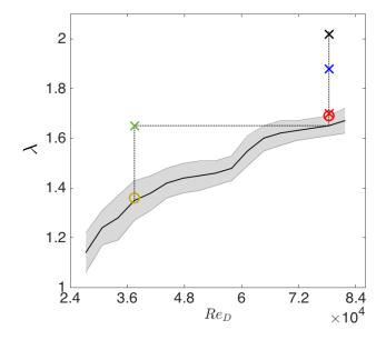
Figure 3.14: Measured turbine operating conditions (symbols) on or above the neutral curve (solid black line) during PIV measurements. Symbols correspond to either flow-driven ('O') or motor-driven ('X') cases. Values for each symbol are given in Table 3.2. Dotted lines are for visual reference only and correspond to the nominal conditions (c.f. Figure 3.12). The shaded region bounds one standard deviation in measured  $\lambda$  along the neutral curve.
