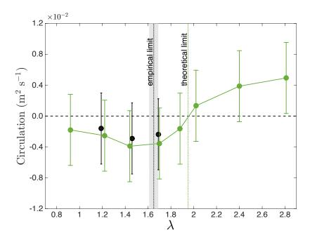
Figure 3.25: Measured circulation for flow-driven (black) and motor-driven (green) cases. Error bars represent an estimate of one standard deviation in measurement error. Motor-driven points are connected with straight line segments.
