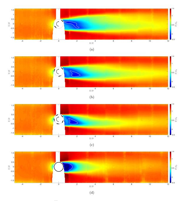
Figure 4.8: Contours of  $\overline{U}/U_0$  measured under load-free conditions for the (a) 2-bladed VAWT, (b) 3-bladed VAWT, (c) 5-bladed VAWT, and (d) cylinder. Airfoil cross-sections for the turbines are drawn to scale.
