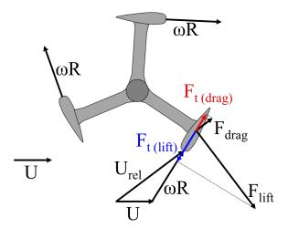
Figure 3.1: Vector diagram of the aerodynamic forces acting on a VAWT airfoil. Here U is the freestream velocity,  $\omega$  is the angular velocity of the turbine, R is the turbine radius,  $U_{\rm rel}$  is the relative freestream velocity as seen by the turbine blade, and  $F_{\rm t(lift)}$  and  $F_{\rm t(drag)}$  are the tangential components of the lift and drag forces, i.e.,  $F_{\rm lift}$  and  $F_{\rm drag}$ , respectively.
