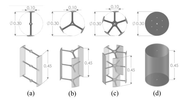
Figure 4.1: Drawings of the (a) 2-bladed VAWT, (b) 3-bladed VAWT, (c) 5-bladed VAWT, and (d) cylinder used for the experiment. Dimensions are in meters.
