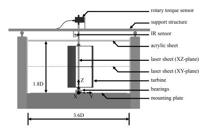
Figure 4.2: Section-view schematic of the experimental setup;  $D=0.3~\mathrm{m}$ .
