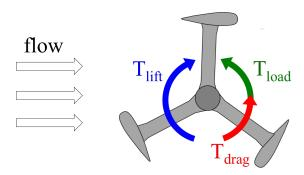
Figure 3.3: Free-body diagram (top view) of a flow-driven VAWT operating with an applied load. Here the net torque due to lift,  $T_{lift}$ , of the blades exceeds the torque due to drag,  $T_{drag}$ , and is balanced by the torque added by an applied load,  $T_{load}$ .
