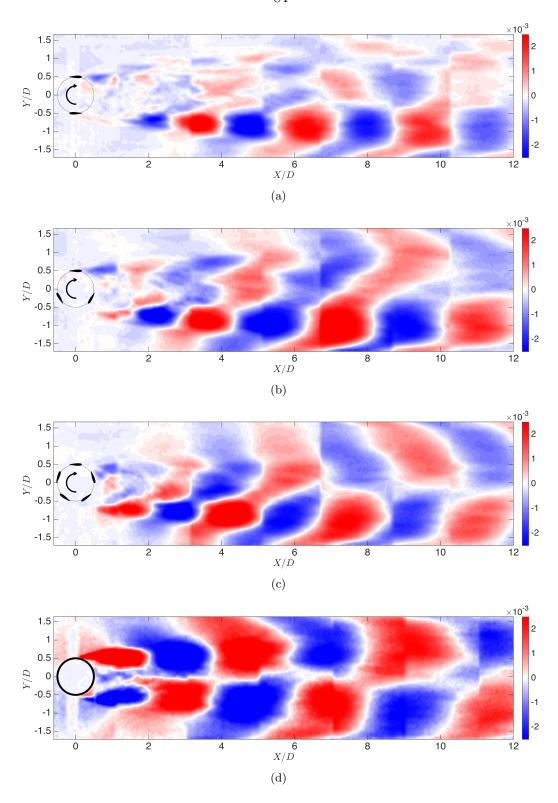
Figure 4.13: Contours of the streamwise component (u') of the dominant POD mode for the velocity fluctuations at the far-wake peak frequency (c.f. Figure 4.10) for the (a) 2-bladed VAWT, (b) 3-bladed VAWT, (c) 5-bladed VAWT, (d) and cylinder. Airfoil cross-sections and angular positions are accurately represented in the figure. The dashed circle in the turbine plots is for reference only and corresponds to the turbine diameter. The solid circle represents the cylinder diameter, D.
