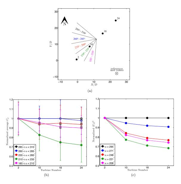
Figure 2.8: The effect of wind direction on turbine performance for the indicated four-turbine array. (a) Schematic of the array with the bins of wind direction. (b) Field measurements of individual turbine performance. Error bars indicate one standard deviation. (c) LRB model prediction of turbine performance for each wind direction, taken as the average in each bin.
