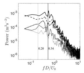
Figure 4.29: Single-point spectra of the velocity fluctuations (v') taken at X/D = 0.9 (——), X/D = 1.7 (---), X/D = 3.3 (----), X/D = 7.3 (-----), and X/D = 10.0 (-----) for the rotating cylinder. The solid vertical line corresponds to the rotation rate of the cylinder, and the dotted vertical line to the shedding frequency of the stationary cylinder.
