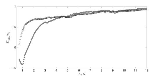
Figure 4.30: Normalized minimum streamwise velocity,  $\overline{U}_{\min}/U_0$ , versus normalized downstream distance, X/D, for the rotating ( $\triangle$ ) and stationary cylinder ( $\bullet$ ).
