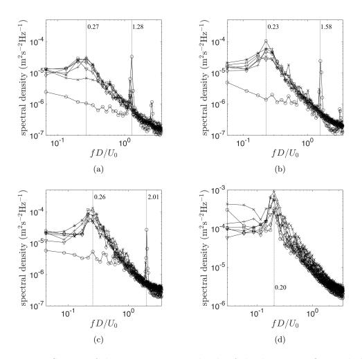
Figure 4.10: Spectra of the time-varying amplitude of the dominant POD mode for the velocity fluctuations under load-free conditions for the (a) 2-bladed VAWT, (b) 3-bladed VAWT, (c) 5-bladed VAWT, and (d) cylinder. The spectra correspond to PIV window 3 ( $\circ$ ), 4 ( $\times$ ), 5 (+), 6 (\*), 7 ( $\square$ ), 8 ( $\diamond$ ) and 9 ( $\bigtriangledown$ ). Dotted vertical lines correspond to the selected near- and far-wake frequencies of the maximum amplitude in the spectra.
