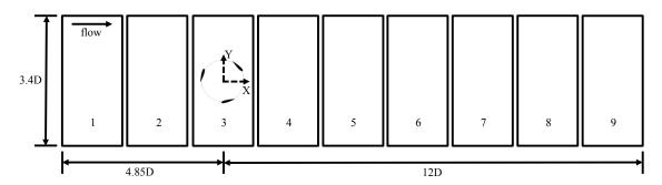
Figure 4.3: Top-view schematic of the nominal turbine position and corresponding PIV windows (1-9) in the XY-plane; D = 0.3 m.
