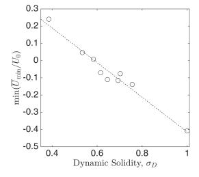
Figure 4.21: Linear correlation ( $R^2=0.96$ ) between the normalized absolute minimum streamwise velocity across the span,  $\min(\overline{U}_{\min}/U_0)$  and the dynamic solidity,  $\sigma_D$ .
