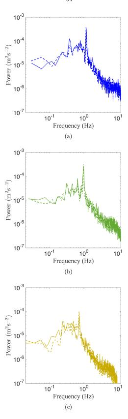
Figure 3.22: Power spectra for the spanwise fluctuating velocity component, v', in flow-driven (solid lines) and motor-driven (dashed lines) cases. Colors correspond to the nominal operating conditions on or below the neutral curve, i.e.,  $\lambda = 1.45$ ,  $Re_D = 7.8 \times 10^4$  (blue),  $6.6 \times 10^4$  (green), and  $5.1 \times 10^4$  (yellow). The measured conditions are given in Table 3.1.
