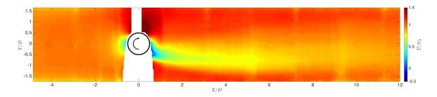
Figure 4.28: Contours of PIV measurements of  $\overline{U}/U_0$  for the cylinder rotating at  $\lambda = 1.69$ .
