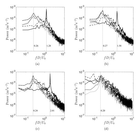
Figure 4.9: Single-point spectra of the velocity fluctuations (v') taken at X/D = 0.9 (——), X/D = 1.7 (---), X/D = 3.3 (----), X/D = 7.3 (-----), and X/D = 10.0 (-----). The spectra correspond to load-free conditions for the (a) 2-bladed VAWT, (b) 3-bladed VAWT, (c) 5-bladed VAWT, and (d) cylinder. Dotted vertical lines correspond to the selected near-and far-wake frequencies of the maximum amplitude in the spectra.
