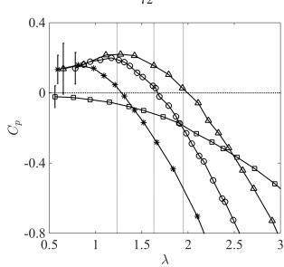
Figure 4.5: Measured values of  $C_p$  for the 2-bladed VAWT ( $\triangle$ ), 3-bladed VAWT ( $\circ$ ), 5-bladed VAWT (\*), and cylinder ( $\square$ ). Error bars indicate one standard deviation in the measured value of  $C_p$ . Dashed vertical lines indicate the 'load-free' PIV measurement conditions for the turbines.
