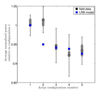
Figure 2.10: Comparison of field measurements and LRB model prediction of average array performance for the five unique configurations of twelve VAWTs. Error bars indicate one standard deviation.
