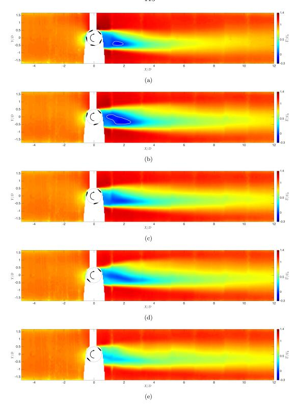
Figure 5.3: Contours of PIV measurements of  $\overline{U}/U_0$  under loaded conditions. The plots are in order from top to bottom with decreasing  $\sigma_D$  (c.f. section 4.3.3) and correspond to the (a) 5-bladed VAWT at  $\lambda=1.01$ , (b) 3-bladed VAWT for  $\lambda=1.41$ , (c) 3-bladed VAWT for  $\lambda=1.20$ , (d) 2-bladed VAWT for  $\lambda=1.61$ , and (e) 2-bladed VAWT for  $\lambda=1.22$ . Airfoil cross-sections for the turbines are drawn to scale.
