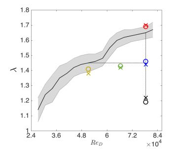
Figure 3.13: Measured turbine operating conditions (symbols) on or below the neutral curve (solid black line) during PIV measurements. Symbols correspond to either flow-driven ('O') or motor-driven ('X') cases. Values for each symbol are given in Table 3.1. Dotted lines are for visual reference only and correspond to the nominal conditions (c.f. Figure 3.11). The shaded region bounds one standard deviation in measured  $\lambda$  along the neutral curve.
