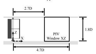
Figure 4.4: Side-view schematic of the PIV measurement window in the XZ-plane; D=0.3 m
