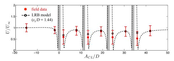
Figure 2.7: Comparison of the LRB model with meteorological tower streamwise velocity measurements for the four-turbine array. Open black circles indicate the LRB model prediction of flow speed at the field measurement locations. Gray rectangles indicate turbine positions.
