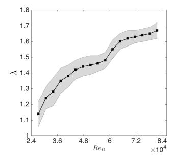
Figure 3.10: Measured values (symbols) of the turbine neutral curve. The shaded region bounds one standard deviation in the measurement of  $\lambda$ . The neutral curve indicates the maximum  $\lambda$  that the turbine could reach for a given  $Re_D$  without an external load applied to its shaft.
