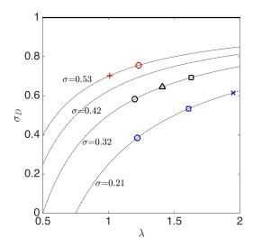
Figure 4.16: Dynamic solidity,  $\sigma_D$ , variation with  $\lambda$  and  $\sigma$ . Measured values are shown with colors and symbols that correspond to the following: the 2-bladed turbine for  $\lambda = 1.95(\times)$ ,  $1.61(\square)$ , and  $1.22(\circ)$ , the 3-bladed turbine for  $\lambda = 1.63(\square)$ ,  $1.41(\triangle)$ , and  $1.20(\circ)$ , the 5-bladed turbine for  $\lambda = 1.23(\circ)$  and  $\lambda = 1.01(+)$ .
