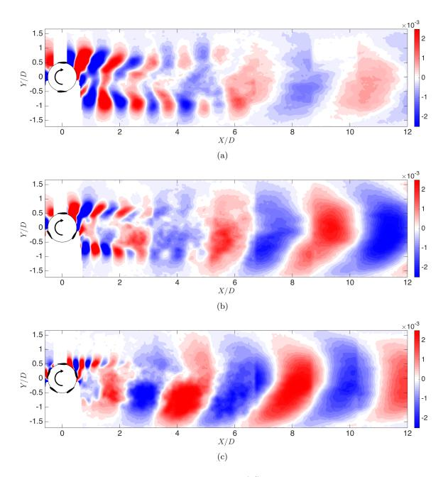
Figure 4.14: Contours of the spanwise component (v') of the dominant POD mode for the velocity fluctuations at both the near and far-wake peak frequencies (c.f. Figure 4.10) for the (a) 2-bladed VAWT, (b) 3-bladed VAWT, and (c) 5-bladed VAWT. In each case,  $\lambda \approx 1.2$ . Airfoil cross-sections and angular positions are accurately represented in the figure. The dashed circle in the turbine plots is for reference only and corresponds to the turbine diameter.
