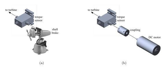
Figure 3.9: Schematic of the setup used for controlling the turbine  $\lambda$  in (a) flow-driven and (b) motor-driven cases.
