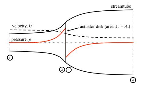
Figure 5.1: Schematic of the flow through a turbine modeled as an actuator disk. The variable streamtube cross-sectional area, velocity, and static pressure fore and aft of the turbine are indicated.
