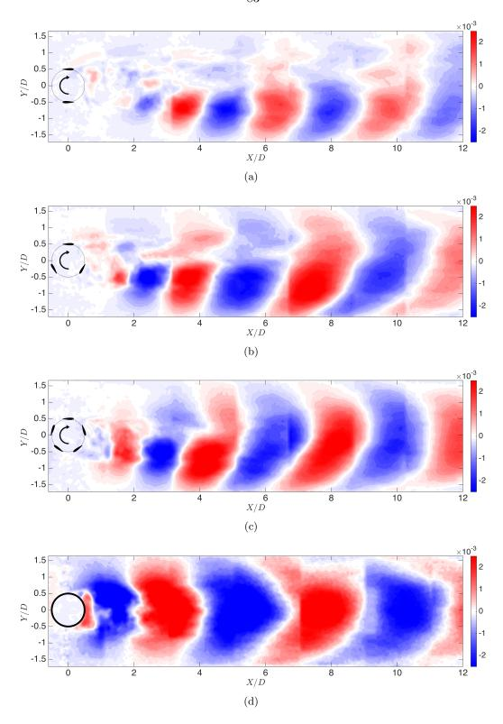
Figure 4.12: Contours of the spanwise component (v') of the dominant POD mode for the velocity fluctuations at the far-wake peak frequency (c.f. Figure 4.10) for the (a) 2-bladed VAWT, (b) 3-bladed VAWT, (c) 5-bladed VAWT, (d) and cylinder. Airfoil cross-sections and angular positions are accurately represented in the figure. The dashed circle in the turbine plots is for reference only and corresponds to the turbine diameter. The solid circle represents the cylinder diameter, D.
