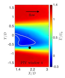
Figure 4.6: Contours of  $\overline{U}/U_0$  for the 3-bladed turbine under load-free conditions ( $\lambda=1.63$ ); the zero-level contour is drawn in white. Measurements correspond to PIV window 4 (c.f. Figure 4.3). The black circle corresponds to the location of the sample time-series in Figure 4.7. Coordinate axes are normalized by the rotor diameter, D.
