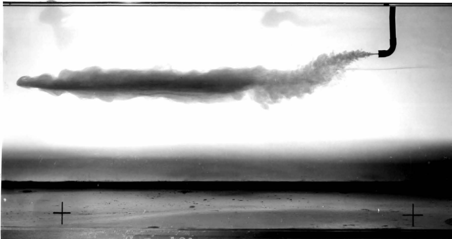
Fig. 20. A horizontal buoyant jet in a stagnant, linearly stratified environment (Jet No. 32, F = 40 and T = 510 , Photo No. 7645.4)
