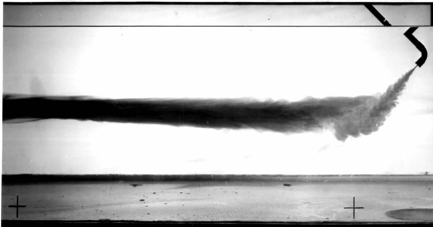
Fig. 21. An inclined ( \theta_0 = 45^\circ ) buoyant jet in a stagnant, linearly stratified environment (Jet No. 18, F = 51 and T = 210 , Photo No. 7642.3)
