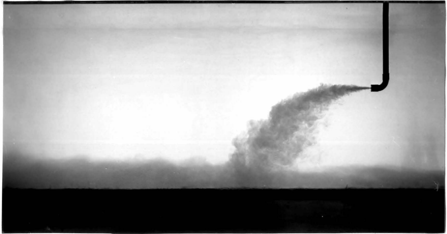
Fig. 28. A horizontal buoyant jet in a stagnant, uniform environment (Jet No. 27, F = 40 , Photo No. 7643-5)
