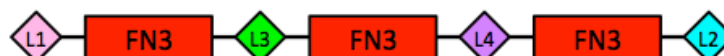
Figure 5-4. Multivalent FN3 construct construction. Each FN3 domain was flanked with a linker for assembly.
