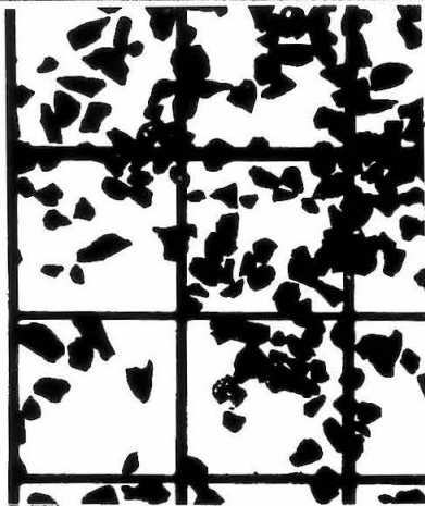
SEDIMENT NO. 10 ILMENITE d_s = 0.112 \text{ mm} , \sigma_g = 1.20 SHAPE : ANGULAR
