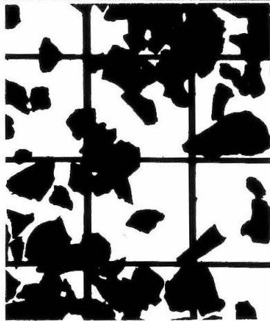
SEDIMENT NO. 13 COAL d_s = 0.258 \text{ mm} , \sigma_g = 1.43 SHAPE : ANGULAR
