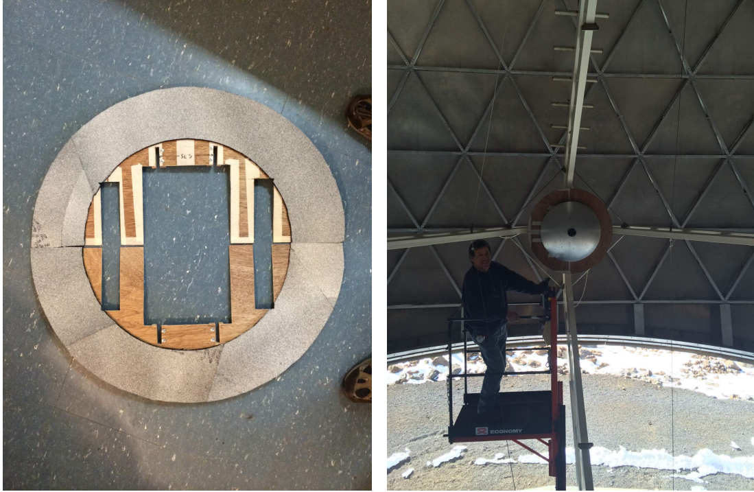
Figure 4.26: Left: The intermediate size (100%) Eccosorb® collar. Right: Steve Baca showing the Eccosorb® collar attached to the secondary mirror of the CSO. Photos taken by Simon Radford.
