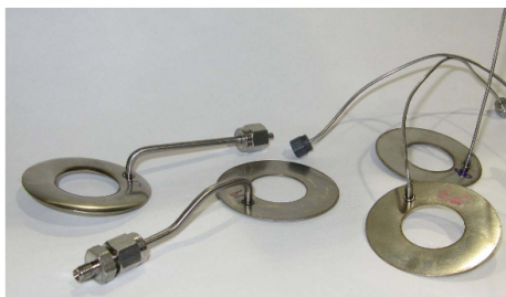
Figure 4.9. Pressure membranes for remote pressure control.
