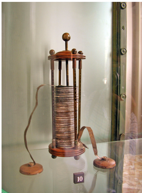
Figure 1.1. Replica of Alessandro Volta's original cell, composed of a stack of zinc and copper disks. Figure: GuidoB- CC BY-SA 3.0
