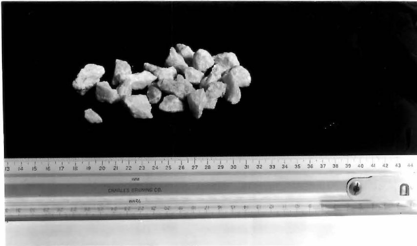
Figure 22. Stone used for bottom roughness in 40-meter flume.
