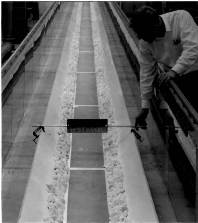
Figure 35. Method of inserting tracer.
