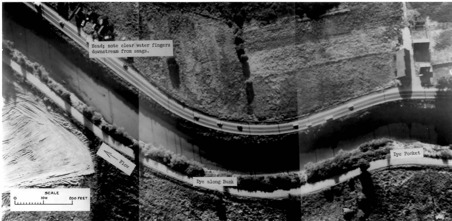
Figure 50. Aerial photograph of dye dispersion, August 17, 0804 hours. Center of cloud approximately 1600 feet downstream from injection point.
