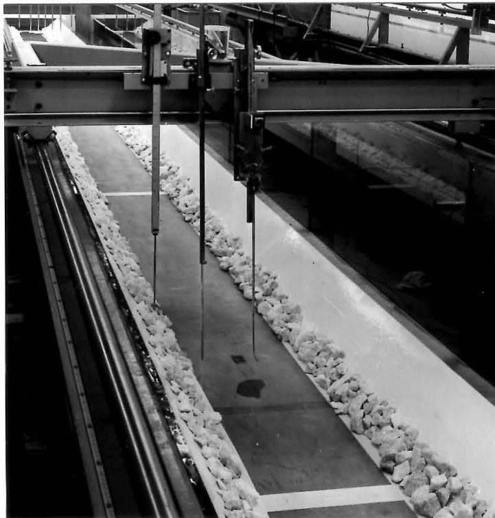
Figure 37. Oblique view of channel for series 2800, 2900, and 3000, showing probe locator pointer, water surface pointer, and Prandtl tube mounted on instrument carriage.
