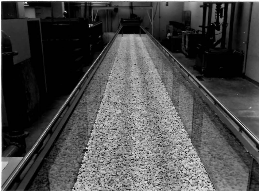
Figure 23. 40-meter flume with stone layer on bottom.
