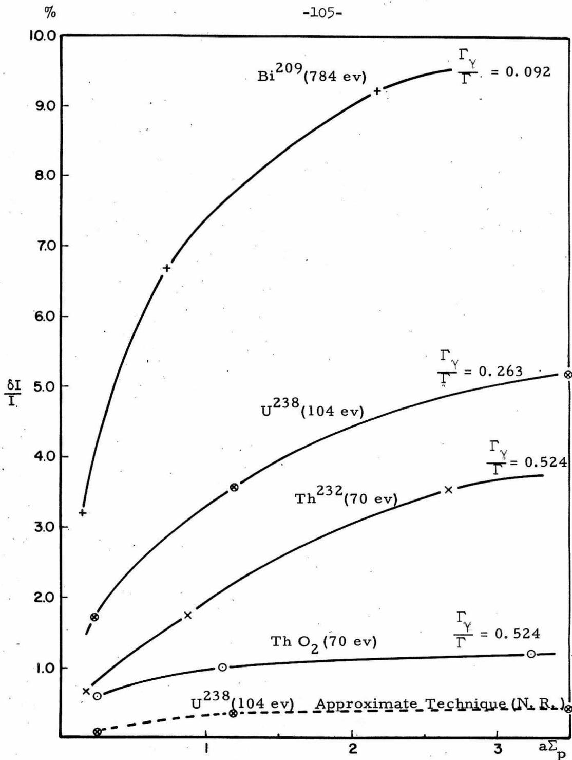
Fig. 21. Fractional error introduced in resonance integral by the flat flux approximation.
