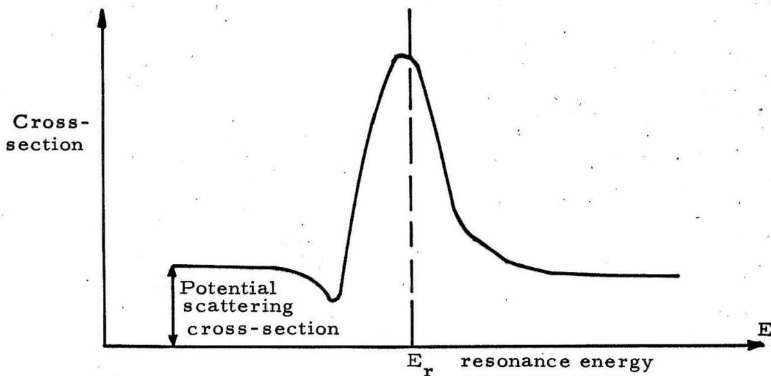
Fig. 1. Schematic illustration of a Breit-Wigner single level line
