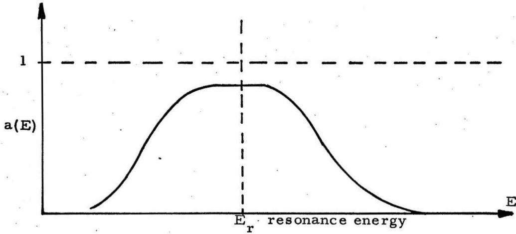
Fig. 3. Schematic illustration of the variation of the absorption probability  $a(E)$  with energy.
