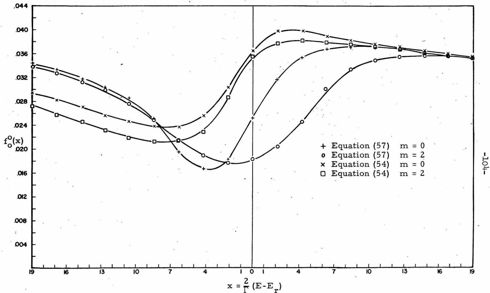
Fig. 20. Solutions for uranium, slab thickness = 7.5 cm.
