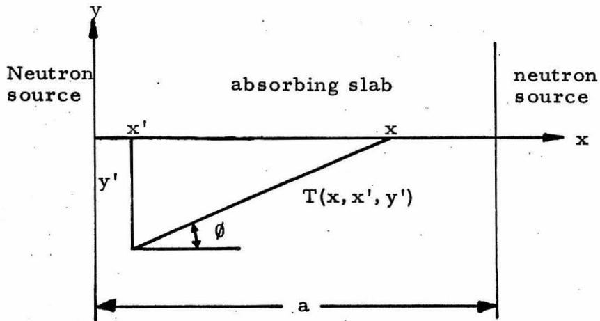
Fig. 4. Slab of absorbing material embedded in a neutron source.
