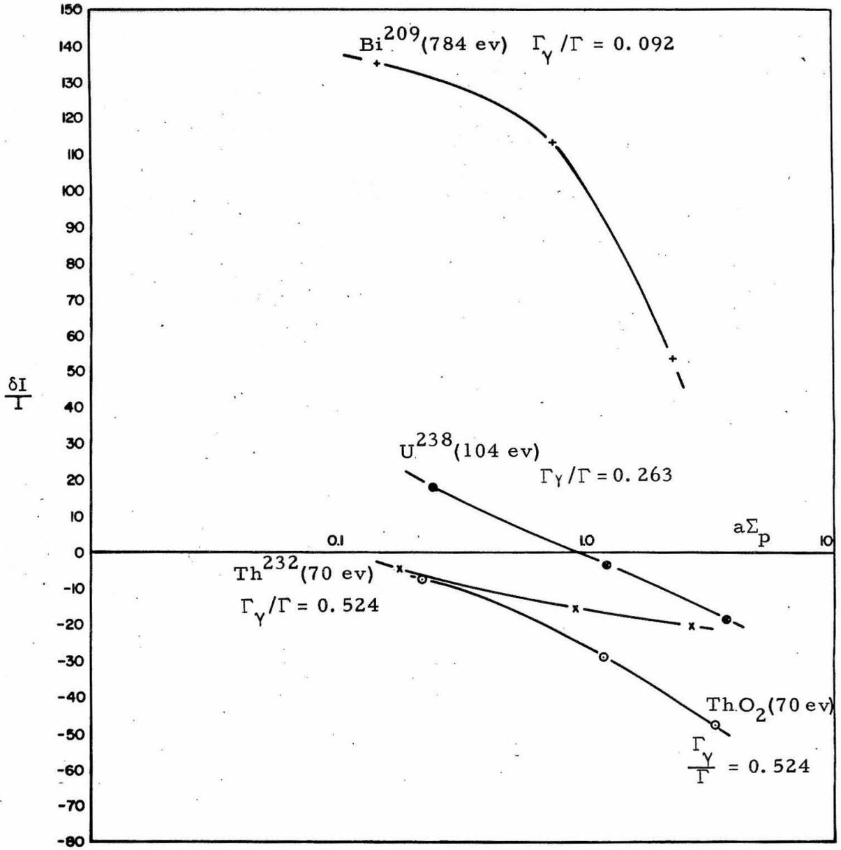
Fig. 23. Fractional error introduced in the resonance integral by the W. R. approximation.
