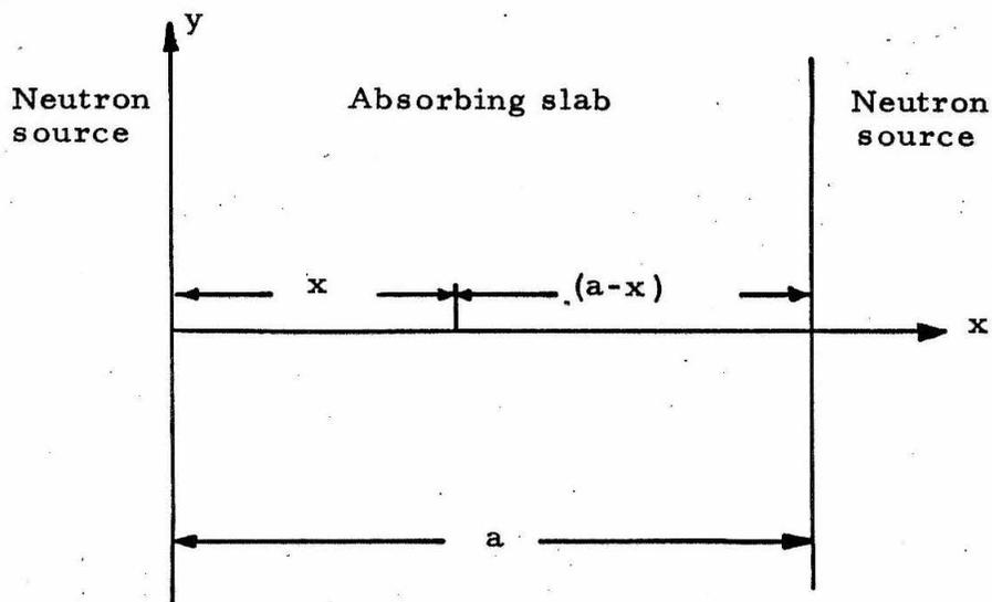
Fig. 2. Absorbing slab surrounded by a neutron source
