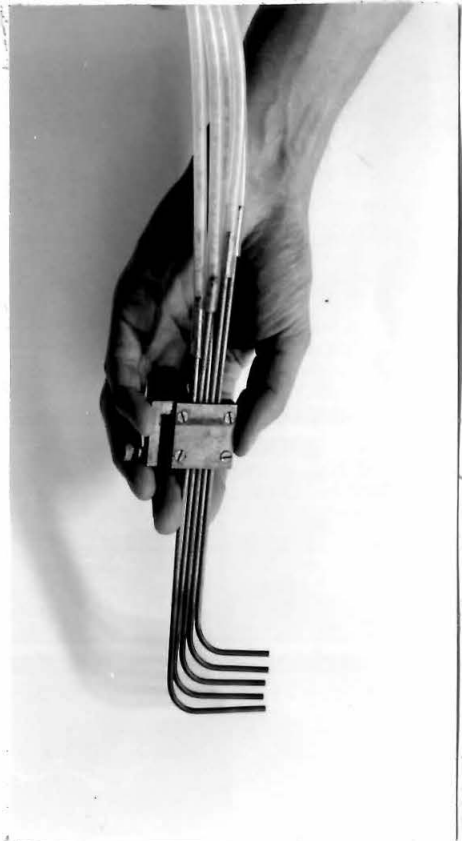
Figure 3.9 A fluid sampling rake.
