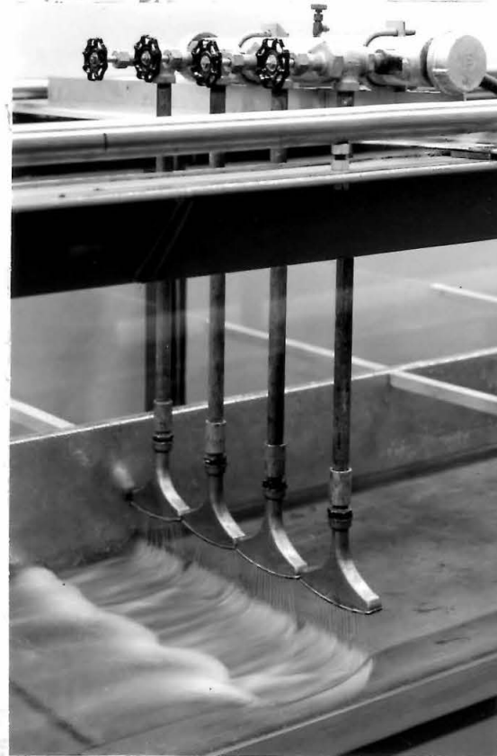
Figure 3.8 The manifold for the wide source.
