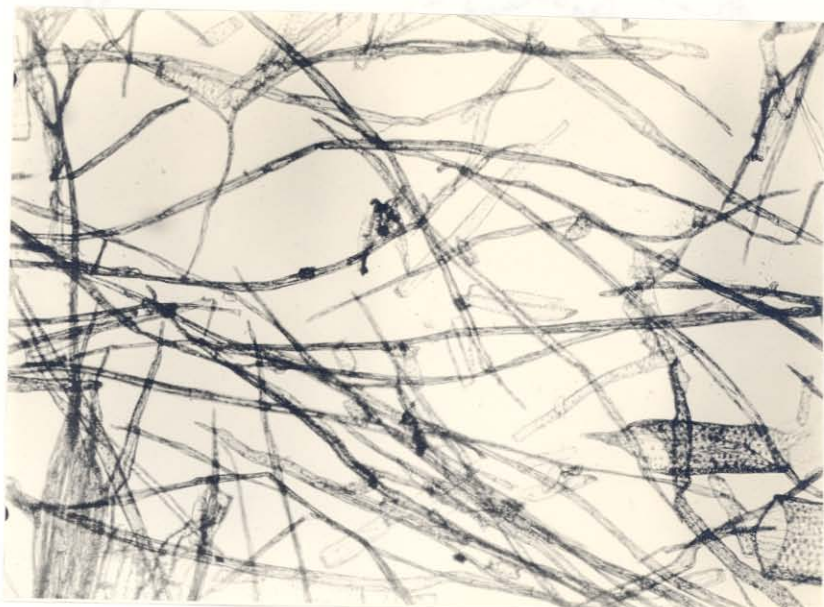
Fig. 4. - Kraft pulp from E. globulus . (Blue Gum.) Cook No. 4. The large, thick cells in the lower, right-hand corner are cells from the vessels. These and the short ray cells contribute no strength to the pulp. Magnification 96 diameters as in Figs. 5, 6, 7, 8 and 9.
