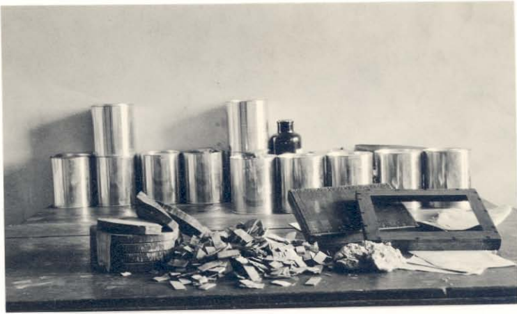
Fig. 1. - Illustrates steps in the process of reducing the wood to chips. The discs first cut from the log and the chips split from them are shown, as well as some of the pulp and a sheet of the paper made on the small hand mold, the two parts of which are shown disconnected.
