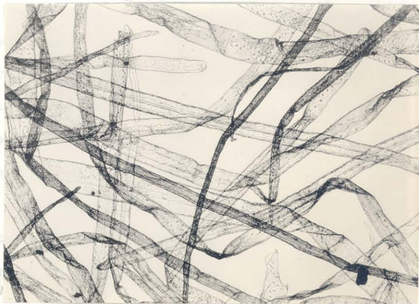
Fig. 9. - Kraft pulp made from red cedar. Shown here enlarged the same as the other photomicrographs for comparison.
