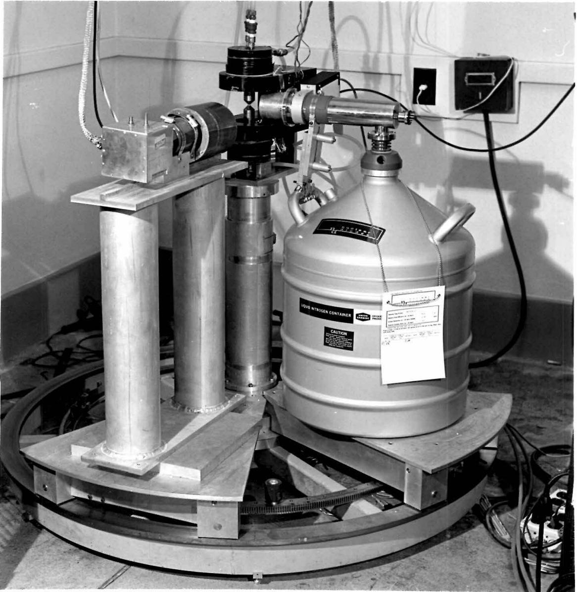
Figure 4: The correlation table with a Ge(Li) detector and a scintillation counter.
