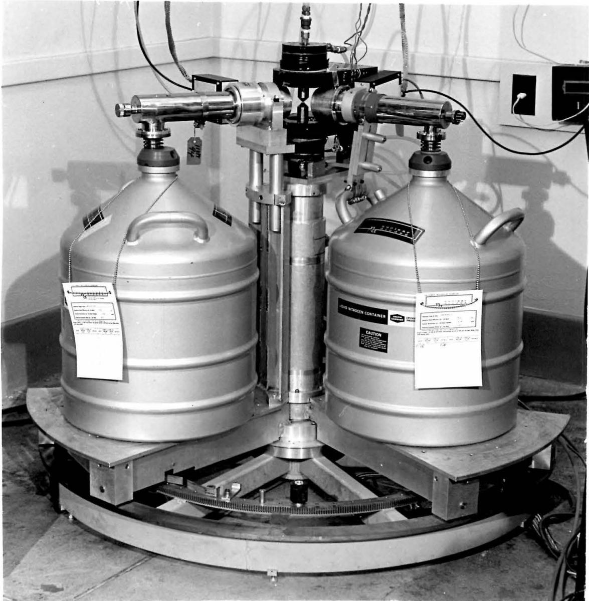
Figure 3: The correlation table utilizing two Ge(Li) detectors. The radioactive source is fixed between the pole tips of the magnet on the center post. The motorized carriage is at left of picture.
