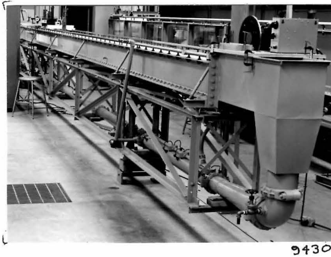
Figure 4.1. The 40-ft tilting flume modified for use as a wave tank.
