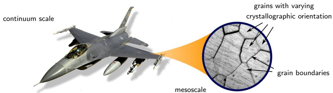
Figure 1.1: Macro- and microscopic view of metal structure. (image credit: imsoup.com, wikipedia.org)
