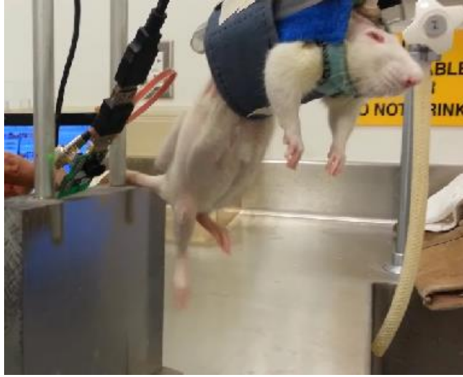
Figure 4.17: Photograph of the wireless implant inducing hindlimb motion in a spinalized rat.
