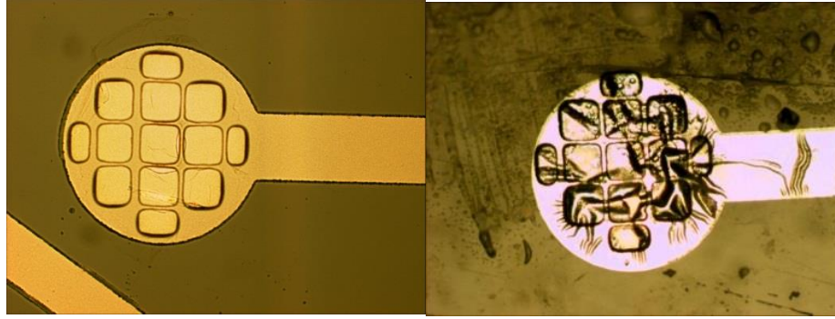
Figure 2.15: Typical electrode before implantation (left) and after explantation (right) when equipped with a grid structure.
