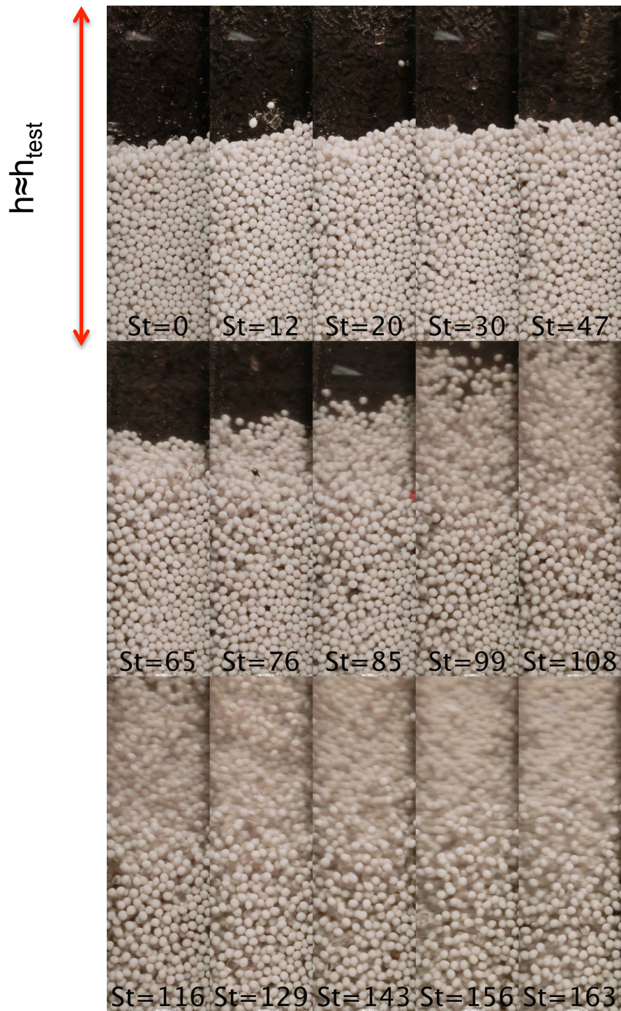
Figure C.18: Image sequence at different Stokes numbers for \bar{\phi} = 40\% . The density ratio is 1.4.
