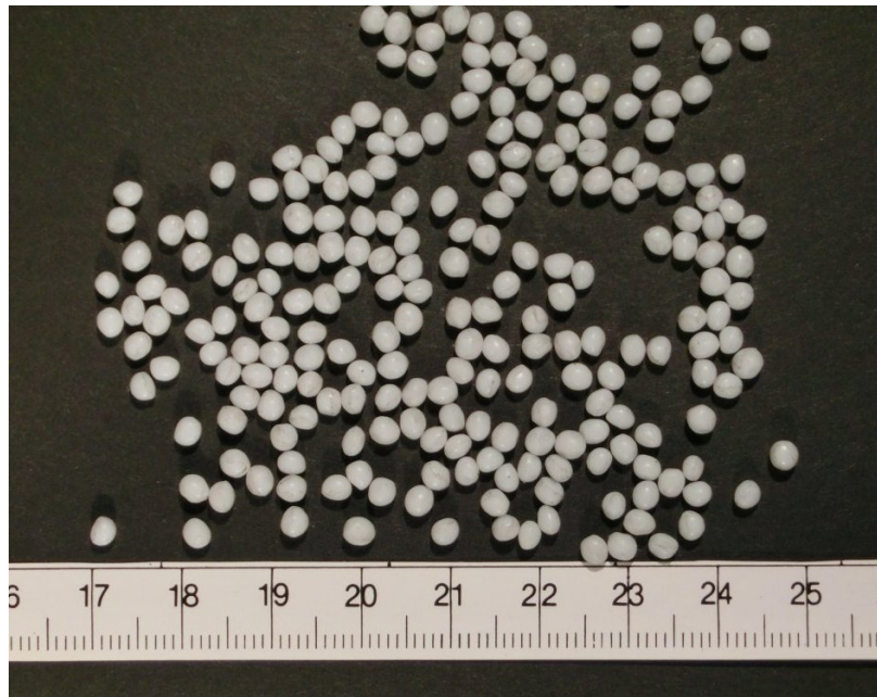
Figure 2.16: Polyester particles. Specific gravity of 1.4 and have an equivalent spherical particle diameter of 2.93 \pm 0.02 mm. Reference shown in cm.
