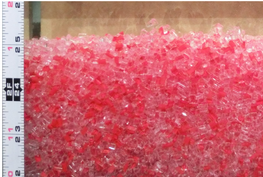
Figure 2.18: Sample of polystyrene particles used for visualization purposes. The particles are immersed in water. The mix of painted particles are evenly mixed with the non-painted ones, and thus the paint does not seem to have a considerable influence on particles density.
