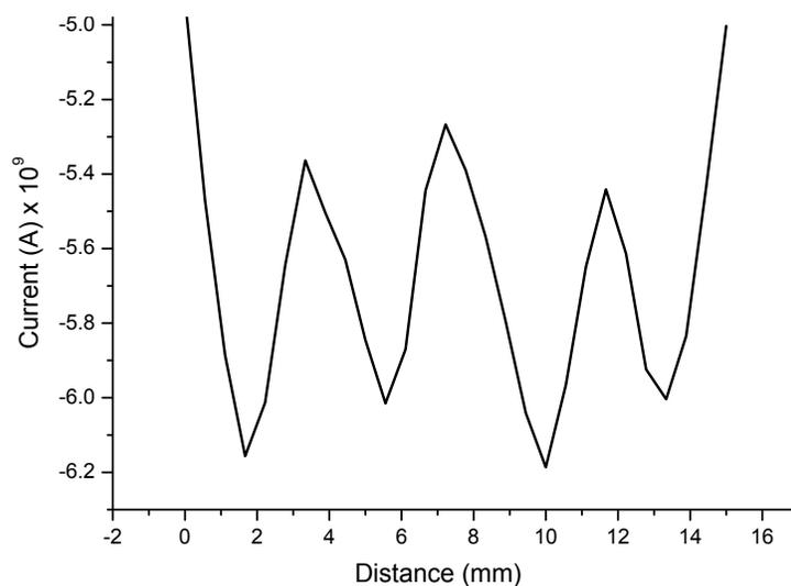
**Figure 3.5** Patterning of a pad containing four strips of well-matched DNA. This was measured in 2  $\mu\text{M}$  methylene blue and 200  $\mu\text{M}$  ferricyanide in Tris buffer (10 mM Tris, 100 mM KCl, 2.5 mM  $\text{MgCl}_2$ , 1 mM  $\text{CaCl}_2$ , pH 7.6). As can be seen, the size and shape of the signals resulting the patterning of the same sequence four times is exceptionally consistent.
