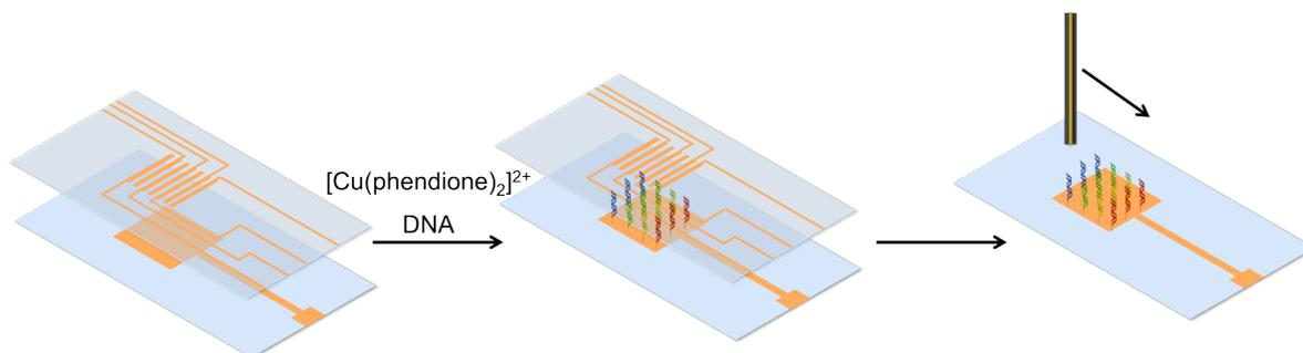
**Figure 3.1** Two working electrode patterning and readout platform. DNA arrays are formed electrochemically through the activation of an inert copper complex to an active catalyst from a secondary set of electrodes. Using the current configuration, up to four individual sequences of DNA are patterned onto a single substrate electrode. Subsequent readout of the sequences on the surface is accomplished by manual scanning of a microelectrode across the secondary electrode.
