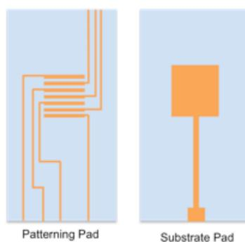
**Figure 3.2** Design for patterning electrodes and substrate electrode. The patterning electrodes pad (*left*) contains four working electrodes that are individually-addressable interspersed with three reference electrodes. The substrate electrode pad (*right*) contains a single, large gold pad and a working electrode contact to the pad.
