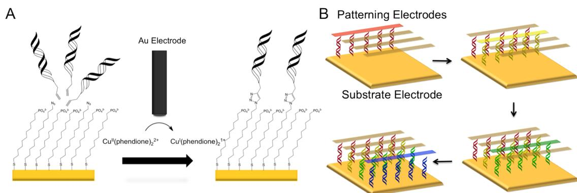
**Figure 3.3** Selective activation for specific covalent attachment of DNA to particular locations. (A) An inert Cu(II) catalyst is electrochemically activated to an active Cu(I) species capable of catalyzing the [3+2] azide-alkyne cycloaddition between alkyne-modified DNA and an azide-terminated thiol monolayer. (B) Up to four different sequences of DNA can be patterned onto a single substrate pad through sequential catalyst activations.
