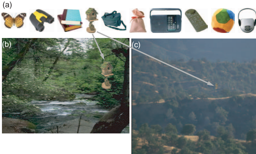
Figure 5.9: (a) Ten of the 21 objects used in the experiment. Each object is scaled such that it consists of approximately 2500 pixels. Artificial pixel and scaling noise is added to every instance of an object before merging it with a background image; (b,c) examples of synthetically generated test images. Objects are merged with the background at a random position by alpha-blending. The ratio of object area vs. image area (relative object size) varies between (b) 5 % and (c) 0.05 %.
