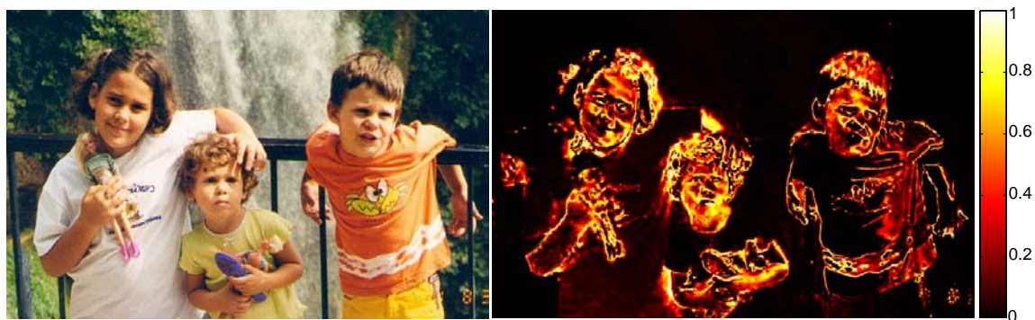
Figure A.7: Example of a color image with faces (left) processed with the skin hue model from eq. A.14, using the parameters from table A.2 (right). The color scale on the right reflects how closely hue matches the mean skin hue, marked with a green cross in figure A.6. Note that face regions show high values, but other skin colored regions do as well, e.g. arms and hands or the orange T-shirt of the boy on the right.
