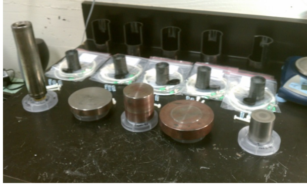
Figure 3.18: Weights applied during glue curing process.
