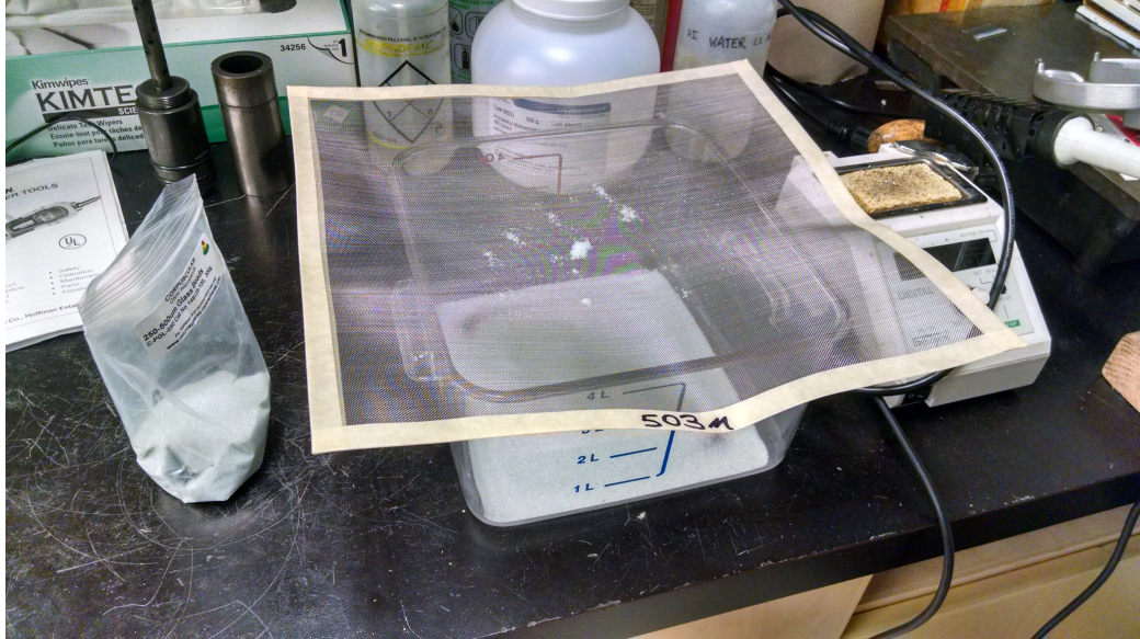
Figure 3.3: Photograph of sieving arrangement for separating particulates from bulk beads.
