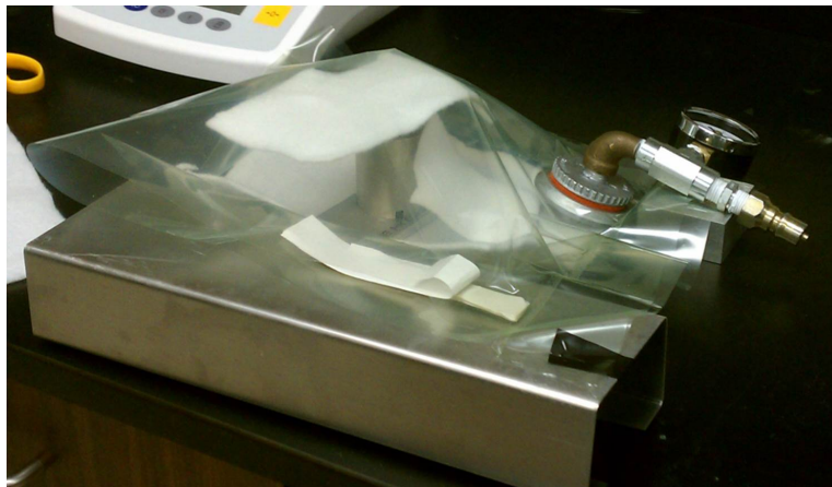
Figure 3.8: Assembled PMMA compression mold in vacuum bag for molding.
