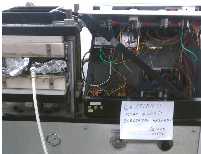
Figure 3.9: Mold under vacuum in press with insulation.
