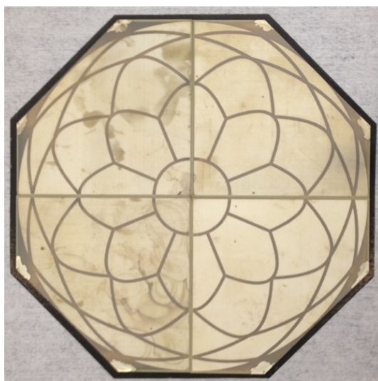
Figure 2.5: Backside of a 150 mm dia. active mirror prototype containing four PZT-5A plates with a custom electrode pattern.
