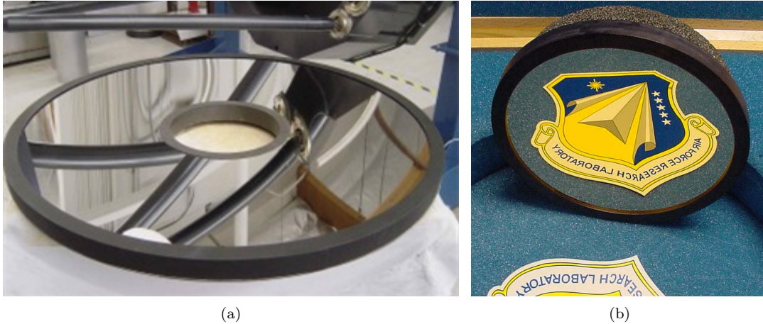
Figure 1.2: a) 1.0 m dia. parabolic composite mirror from Composite Mirror Applications [6]. b) 150 mm. dia. CFRP mirror with a reflective nanolaminate facesheet [7].
