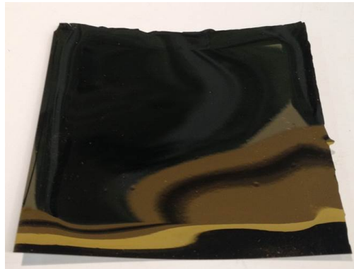
Figure 5.4: Top-view of CFRP + nanolaminate facesheet after a thermal co-cure displaying significant thermal distortions.
