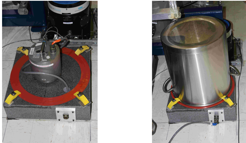
Figure E.2: Guralp seismometer installed in the seismic isolation kit with internal cabling.
