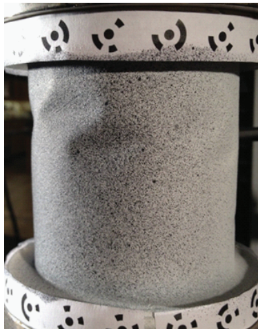
Figure 4.25: Typical buckling shape for circular shells.
