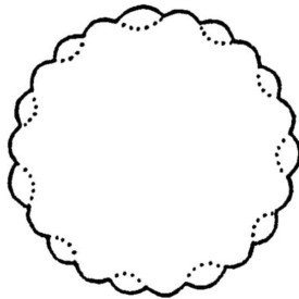
Figure 2.6: Cross-sections of dominant eigenmode of circular shell (solid and dashed arcs) and Aster shell (solid line) with R/t = 490 .
