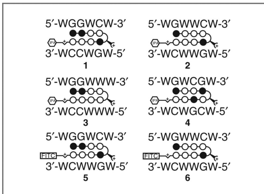
Figure 3.1 Ball-and-stick models of polyamides 1 to 6 with DNA target sequences as follows: 1, 5'-WGGWCW-3'; 2, 5'-WGWWCW-3'; 3, 5'-WGGWWW-3'; 4, 5'-WGWCGW-3'. Polyamides 5 and 6 are FITC-analogs of polyamides 1 and 2, respectively, used for fluorescence microscopy experiments. Chemical structures of polyamides 1 to 6 are in Fig. 3.2. IPA, isophthalic acid.
