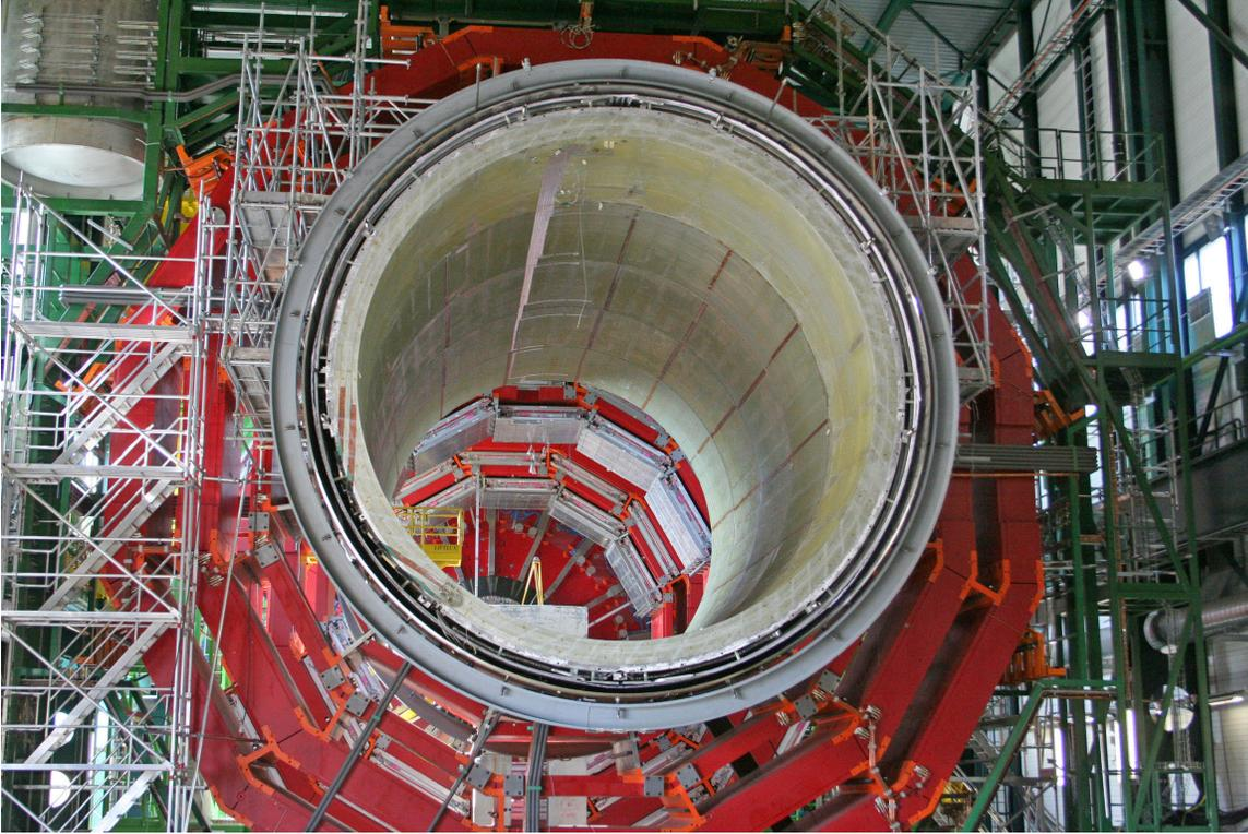
Figure 3.3: The assembly of the yoke.
