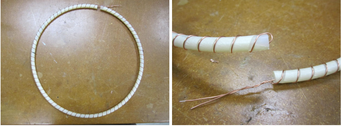
Figure H.1: Photos of the Rogowski coil before it was enclosed in heat shrink.
