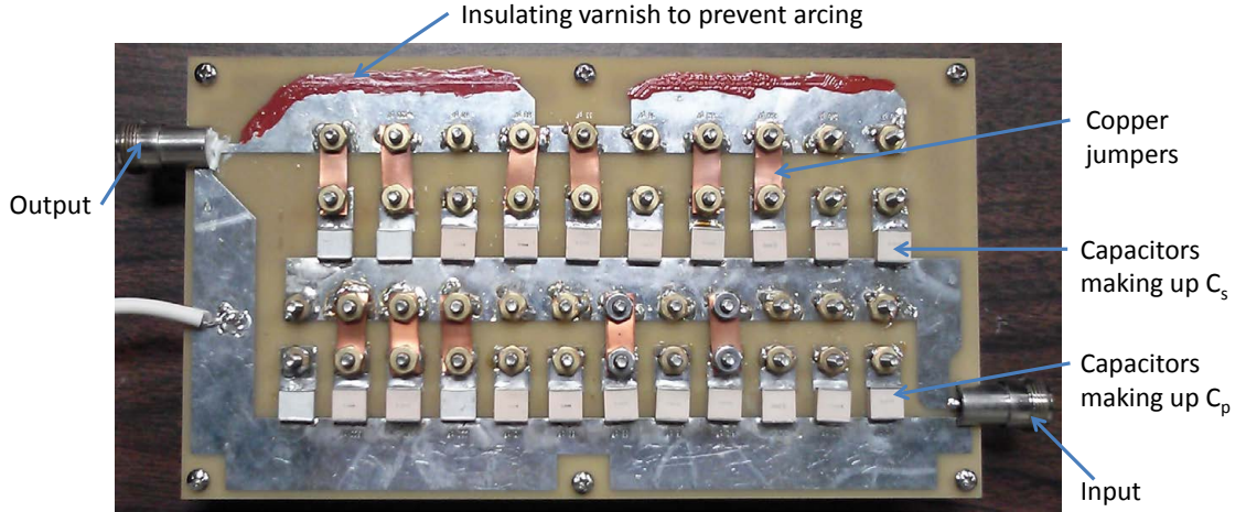
Figure 2.10: Binary arrays of capacitors used to implement the variable capacitors C_p and C_s for the matching circuit. Removable copper jumpers were used to connect the desired capacitors into the circuit.
