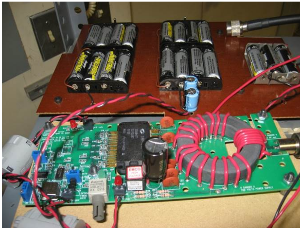
Figure 2.5: Photo of 3 kW RF amplifier, which was mounted on a 3" x 7.5" printed circuit board, and the AA batteries that powered it. The wires connecting the batteries to the board were twisted and passed through ferrite RF chokes to reduce interference between the amplifier's high voltage output stage and low voltage pulse generation stage.
