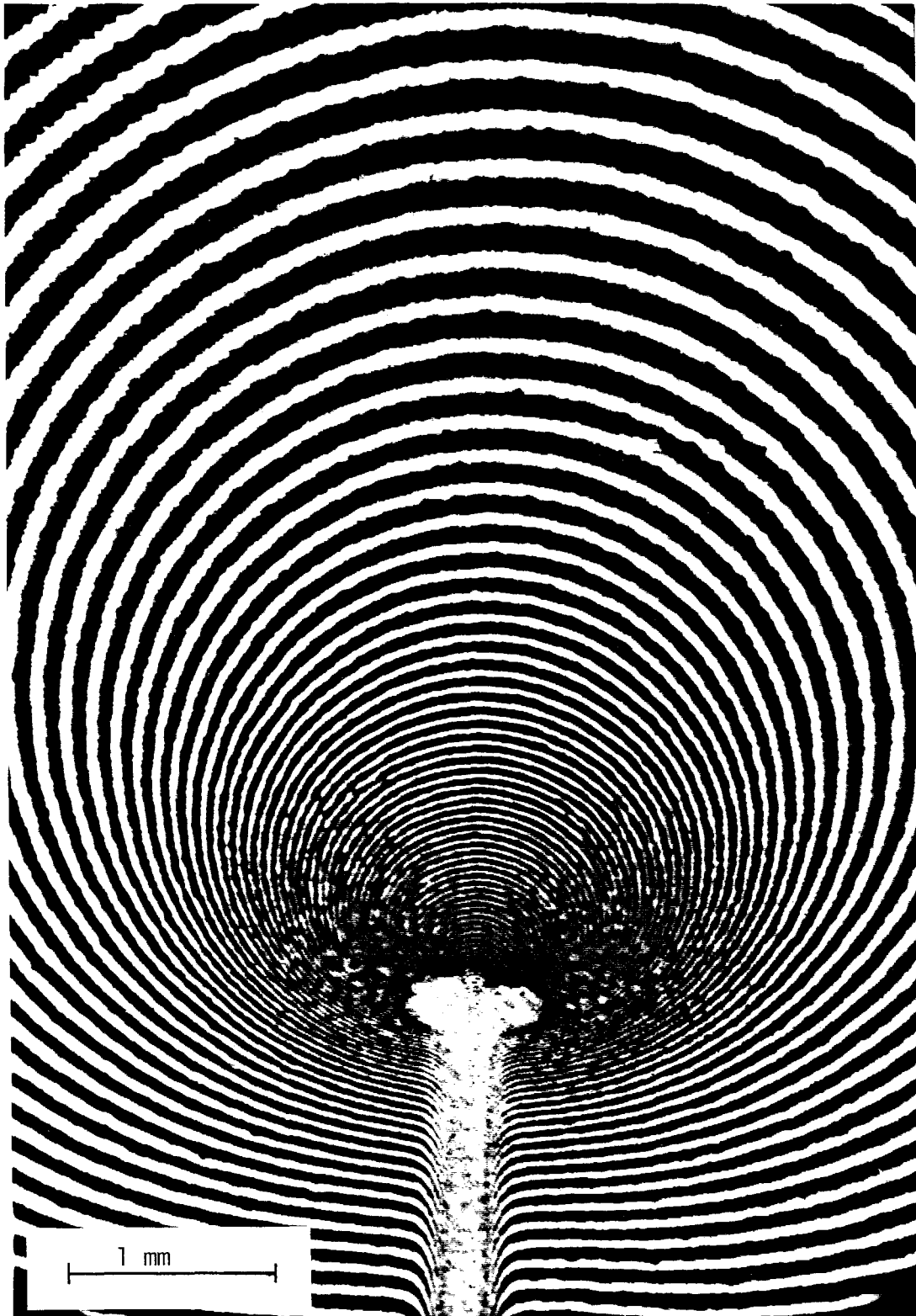
Figure 5.13 Enlargement of crack tip region, 35000 N. Contrast is reverse of Figures 5.11 and 5.12.
