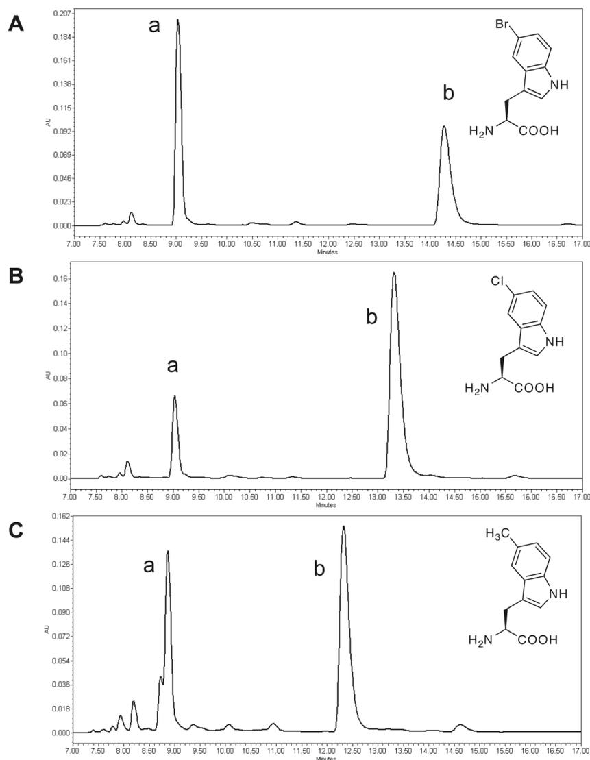
**Figure 2-10.** HPLC analysis of the transfer of tryptophan analogs **15**, **16**, and **17** to KA-AMC by the L,F-transferase. A) Analysis of the transfer of **15** after charging by the T415G yeast PheRS. B) Analysis of **16** after charging by the T415G yeast PheRS. C) Chromatograph showing transfer of **17** to KA-AMC after charging by the T415G yeast PheRS. In All traces, peak **a** is KA-AMC and peak **b** is the tripeptide product.
