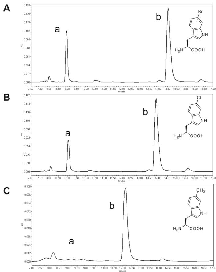
**Figure 2-11.** HPLC analysis of the transfer of tryptophan analogs **18**, **19**, and **20** to KA-AMC by the L,F-transferase. A) Analysis of the transfer of **18** after charging by the T415G yeast PheRS. B) Analysis of **19** after charging by the T415G yeast PheRS. C) Chromatograph showing complete transfer of **20** to KA-AMC after charging by the T415G yeast PheRS. Peak **a** is KA-AMC and peak **b** is the tripeptide product.
