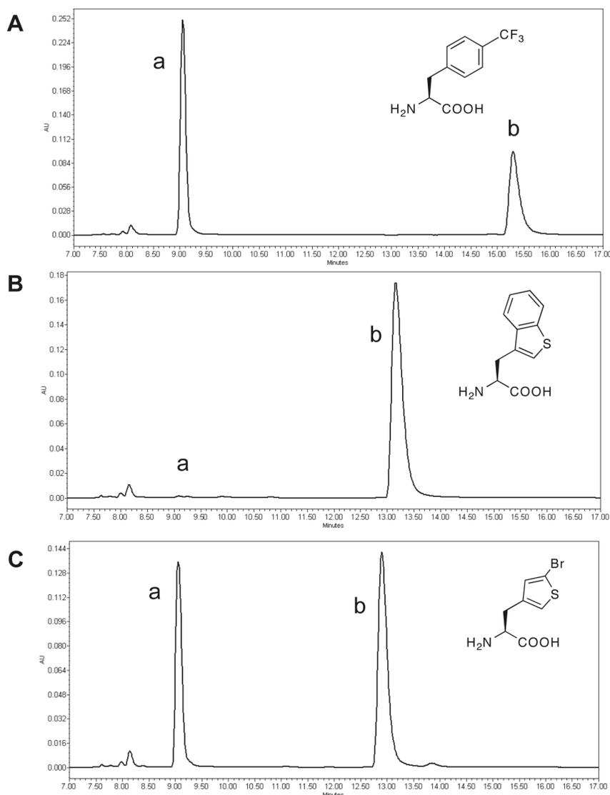
**Figure 2-9.** HPLC analysis of the transfer of tryptophan analogs **12**, **14**, and **11** to KA-AMC. A) Analysis of the transfer of **12** to KA-AMC after charging by the T415G yeast PheRS. B) HPLC Analysis of the complete transfer of **14** to KA-AMC after charging by the T415G yeast PheRS. C) Analysis of the transfer of **11** to KA-AMC after charging by the T415G yeast mutant PheRS. In all traces, peak **a** is KA-AMC and peak **b** is the tripeptide product.
