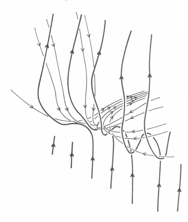
Schematic representation of a plane interface between a uniform magnetic field and a magnetic field with a neutral point. This field configuration is essentially the same as that shown in figure C-1, while the geometry is greatly simplified.
