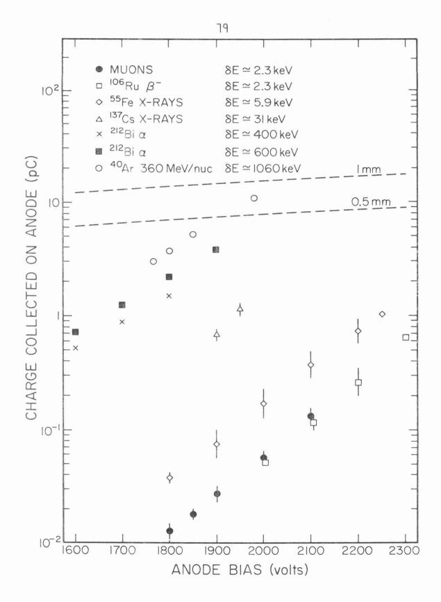
avalanche is comparable to this static charge, a reduction in the gain of the chamber is expected since the charge in the electron cloud reduces the electric field seen by late arriving electrons.
