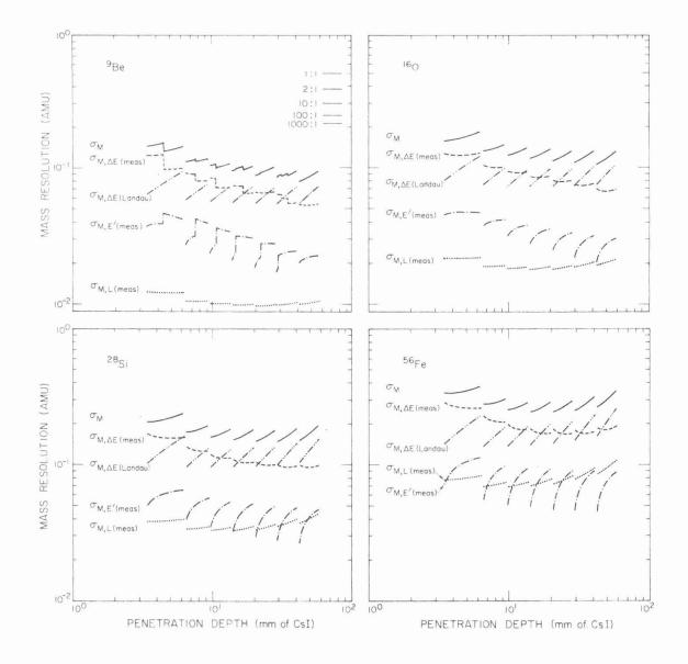
Landau fluctuations, thickness uncertainties, and uncertainties in the measurements of  $\Delta E$  and E' are shown. Tick marks on the right hand sides of these plots indicate the mass resolution required to obtain an inflection point between Gaussian distributions whose centers are separated by [ AMU for various abundance ratios.
