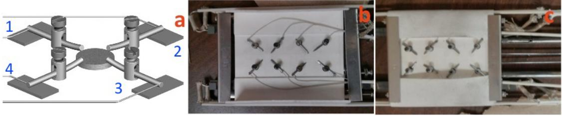
Figure 2.2: Resistivity and Hall coefficient were measured by the four point Van der Pauw method. Image courtesy of Heng Wang.
