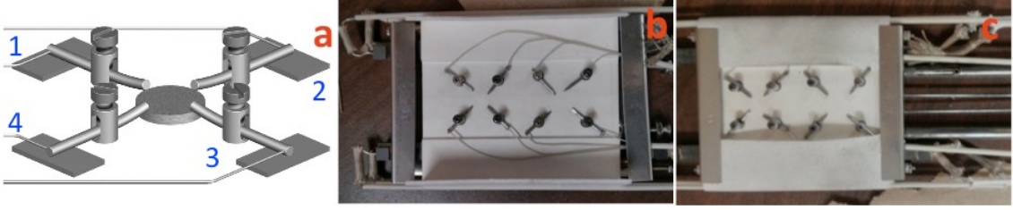
Figure 2.2: Resistivity and Hall coefficient were measured by the four point Van der Pauw method. Image courtesy of Heng Wang.
