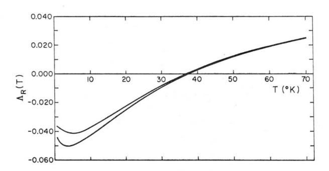
Fig. 3. Real part of the self-energy for anti-ferromagnetic coupling, J=-0.021 ev, ρ = (10/10π) atom level. The lower curve corresponds to Fermi energy while the upper curve is evaluated for x = 0.001 ev, being measured from Fermi energy.
