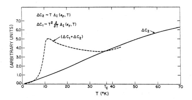
Fig. 13 Incremental specific heat as a function of temperature.  $\Delta C_1$  and  $\Delta C_2$  correspond to the contributions of the two terms of equation (IX. 12).  $\Delta C_1$  curve has been greatly exaggerated for the sake of clarity.
