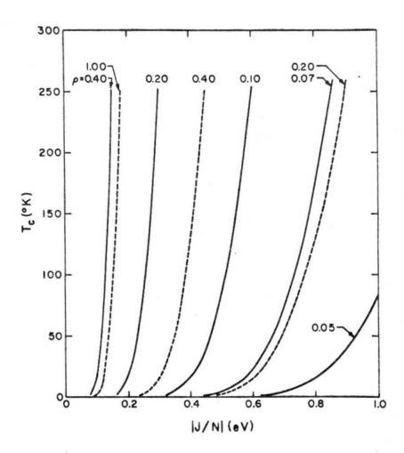
Fig. 10 Critical temperature against exchange interaction strength. Solid and dashed curves correspond to J < o and J > o respectively.
