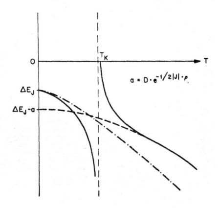
Fig. 2. Energy shift (or Free Energy shift) as a function of temperature. Solid line represents the case J < o. Dashed curve represents the conjectured behaviour for J < o, going to (ΔE<sub>J</sub>-a). The dash-dot curve represents the case J > o. ΔE<sub>J</sub> is the perturbation theory result for energy shift.
