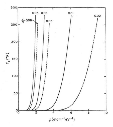
Fig. 12 Critical temperature against the density of states of the host. Solid and dashed curves correspond to J < o and J > o respectively.
