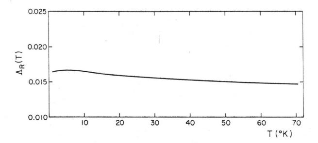
Fig. 7 Real part of self-energy for ferromagnetic coupling using the same magnitude of J = 0.021 ev as for antiferromagnetic coupling shown in Fig. 3. Note the absence of a critical temperature down to 1°K.
