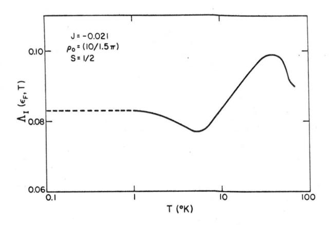
Fig. 14.  $\bigwedge_{I}(\mathcal{E}_{F}, T)$  plotted against temperature on logarithmic scale. Note the linear dependence for 0.3  $T_{c} \le T \le 0.6 T_{c}$  where  $T_{c}$  is around 40°K.
