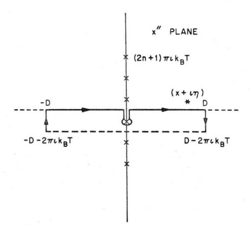
Fig. 15 Contour of integration for (A3), dashed line and the deformed contour, solid line. The x 's are the poles of the integrand.
