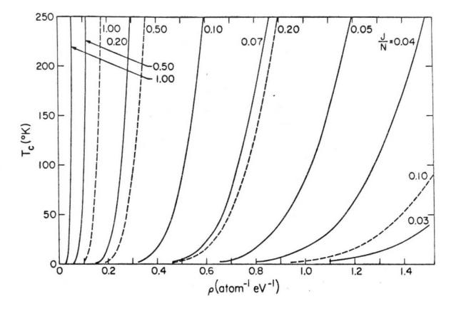
Fig. 11 Critical temperature against the density of states of the host. Solid and dashed curves represent the cases J < o and J > o respectively.
