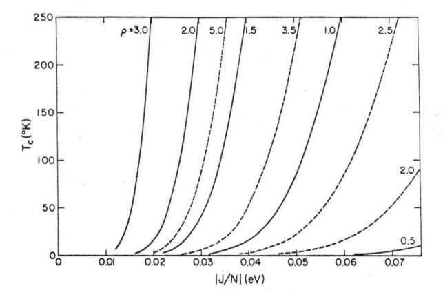
Fig. 9 Critical temperature plotted against exchange interaction strength. Solid curves correspond to J < o and dashed curves to J > o.
