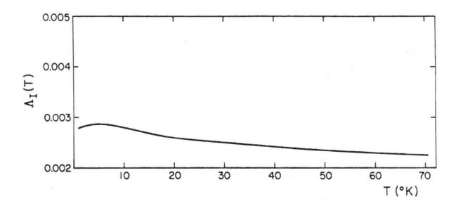
Fig. 8 Imaginary part of self-energy for ferromagnetic coupling using the same magnitude of J = 0.021 ev as for antiferromagnetic coupling shown in Fig. 5.
