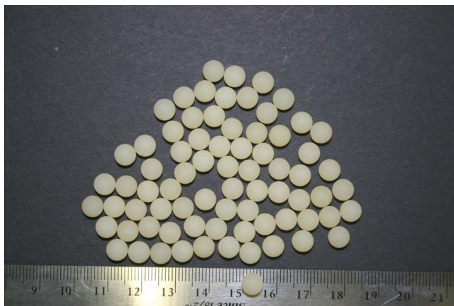
Figure 3.15. The nylon spheres as used in the rheological experiments. The spheres have a specific gravity of 1.15 and have an equivalent spherical particle diameter of 6.36 \pm .02 mm. The ruler shown for reference measures in centimeters.
