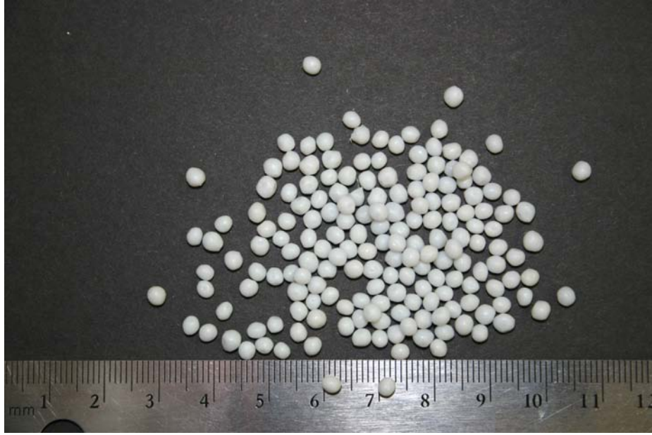
Figure 3.17. The polyester scalene ellipsoids as used in the rheological experiments. The ellipsoids have a specific gravity of 1.40 and have an equivalent spherical particle diameter of 2.93 \pm .02 \text{ mm} . The ruler shown for reference measures in centimeters.
