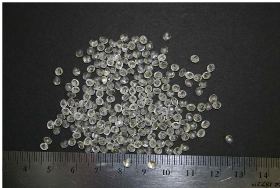
Figure 3.21. The SAN scalene ellipsoids as used in the rheological experiments. The ellipsoids have a specific gravity of 1.07 and have an equivalent spherical particle diameter of 3.22 \pm .02 mm. The ruler shown for reference measures in centimeters.
