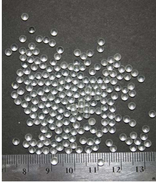
Figure 3.13. The glass spheres as used in the rheological experiments. The spheres have a specific gravity of 2.52 and have an equivalent spherical particle diameter of 3.04 \pm .04 mm. The ruler shown for reference measures in centimeters.
